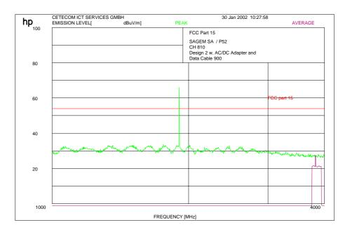
Peak at 1909.8 MHz shows the carrier frequency suppressed by narrow band rejection filter
