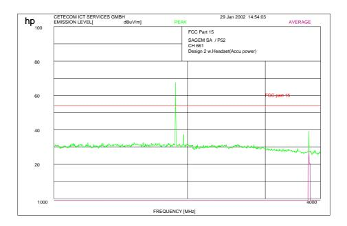
Peak at 1880.2 MHz shows the carrier frequency suppressed by narrow band rejection filter
