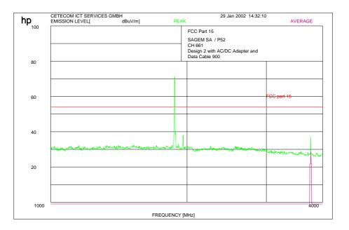
Peak at 1880.2 MHz shows the carrier frequency suppressed by narrow band rejection filter
