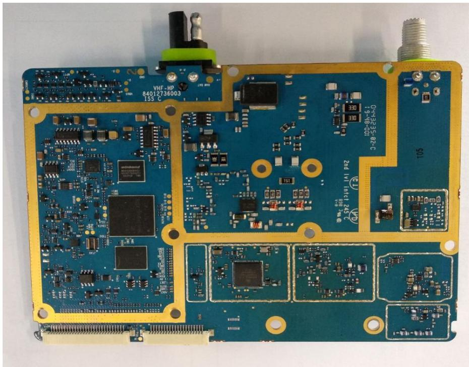
RF board without Shields (Bottom)
