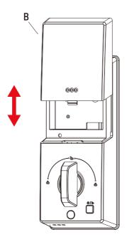
This Electronic lock requires (4) High Quality AA Alkaline batteries. When all 4 batteries are installed in the correct position, you should hear 2 beeps and the keypad will illuminate.
