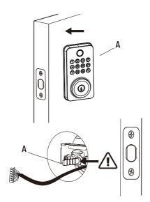
Check that the Rubber Gasket is secured on the Exterior Assembly. Insert the Exterior Assembly onto the door with the tailpiece going through the Deadbolt Latch Set in the VERTICAL POSITION. Route the Control Wire through the door under the Deadbolt Latch Set.
