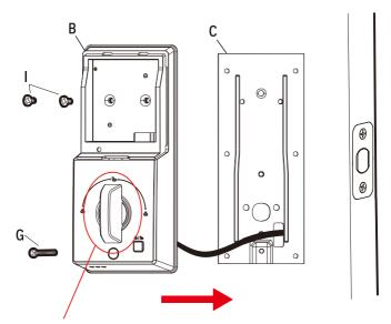
The knob must be twisted to the vertical state
