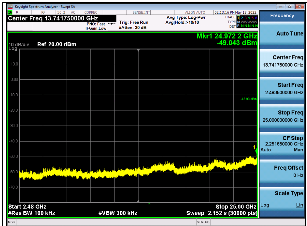
Test_Graph_EDR_ANT1_2402_3Mbps_Higher Band Emissions
