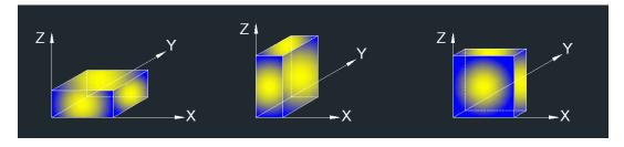
Note 1: For all radiated test, EUT in each of three orthogonal axis emissions had been tested, but only the worst case (X axis for Upward Radar, Z axis for Forward Radar, Z axis for Simultaneously Transmission) data recorded in the report.
