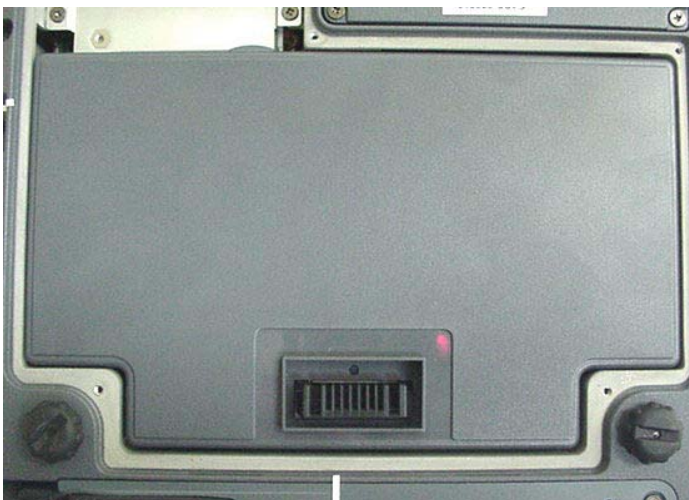
Internal Lithium-ion Battery (Model: T8M-E)
