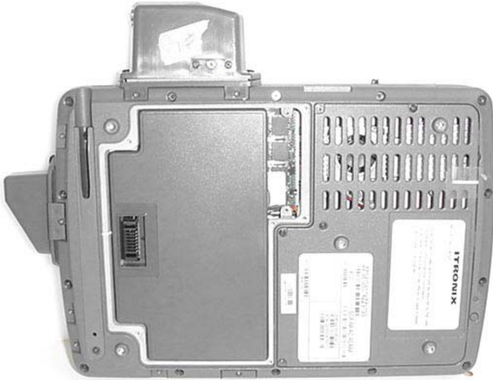
IX325 with Internal Lithium-ion Battery (Model: T8M-E)
