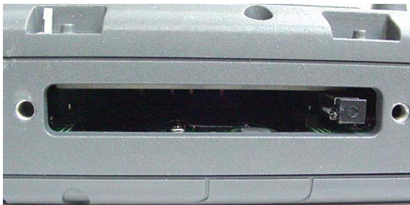
IX325 PCMCIA Card Slot (AirCard 580 Removed)
