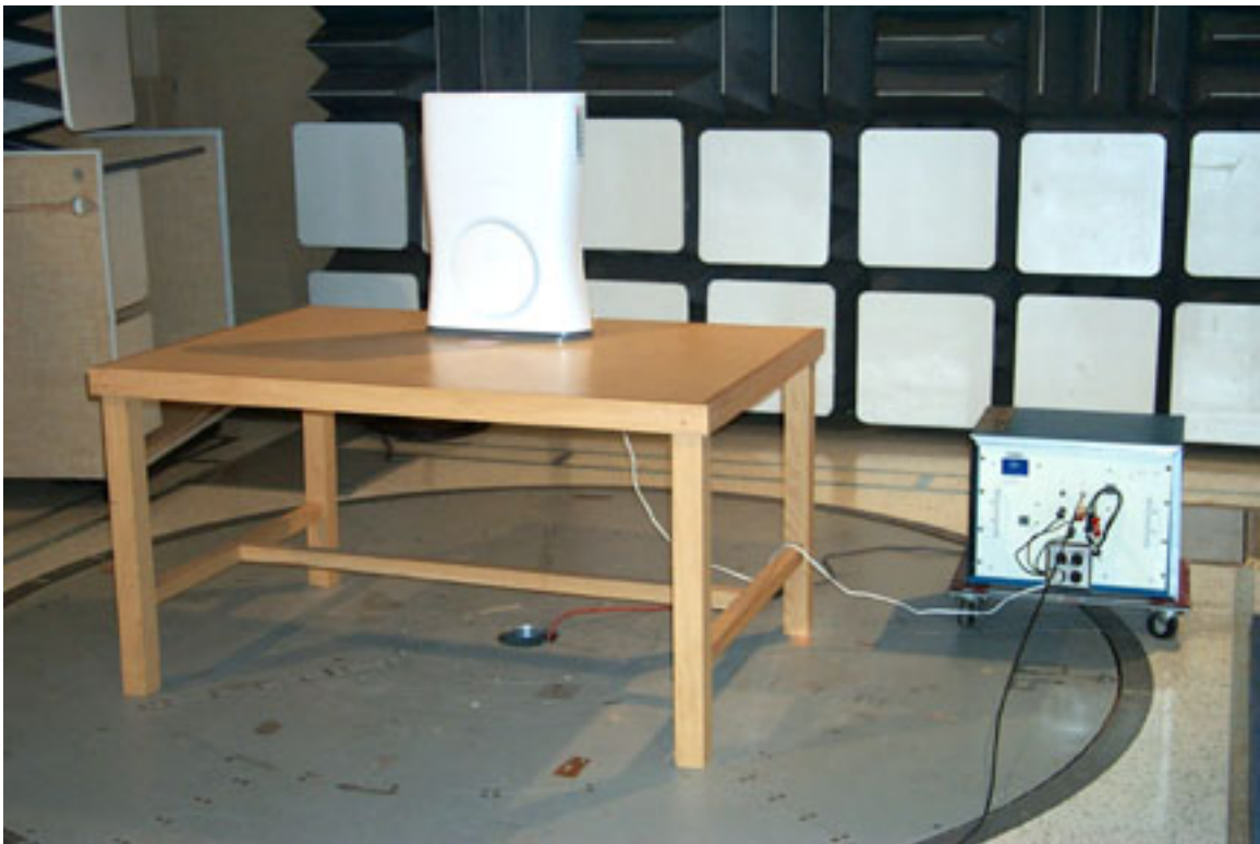
Conducted Emissions Test Setup (Ionizer)
