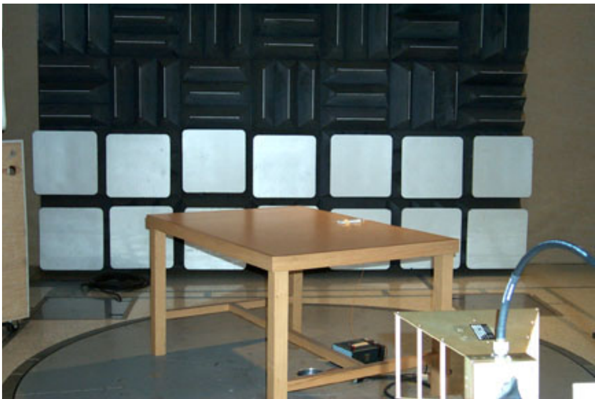
Conducted Emissions Test Setup (Remote)
