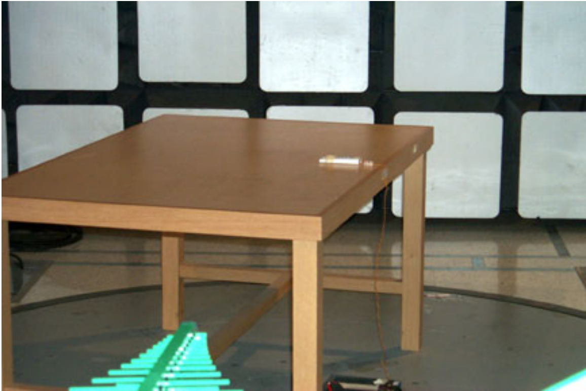
Radiated Emissions Test Setup (Remote)
