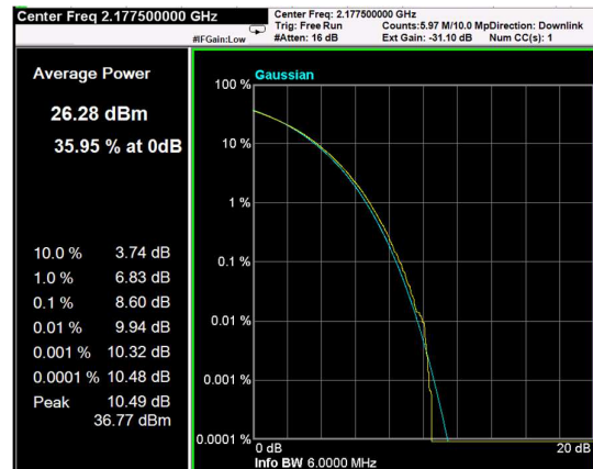
Channel: TOP, Modulation: QPSK, BW=5MHz, CCDF
