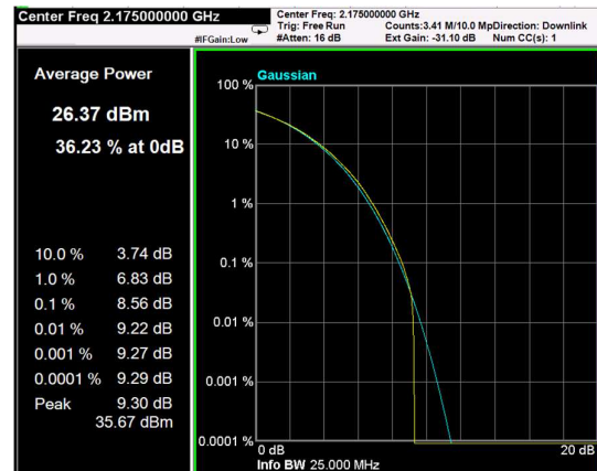
Channel: TOP, Modulation: QPSK, BW=10MHz, CCDF
