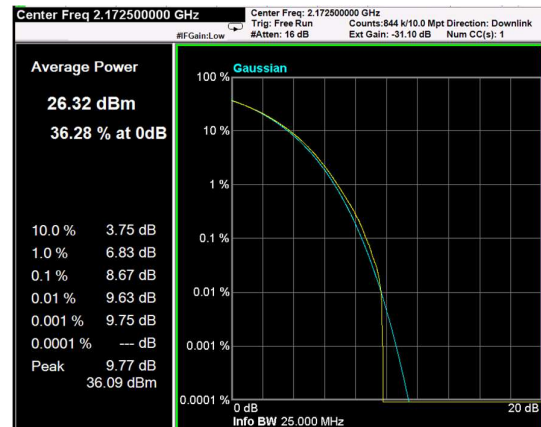
Channel: TOP, Modulation: QPSK, BW=15MHz, CCDF
