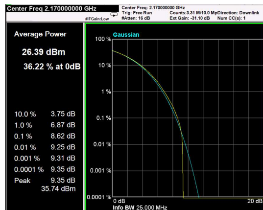
Channel: TOP, Modulation: 256QAM, BW=20MHz, CCDF
