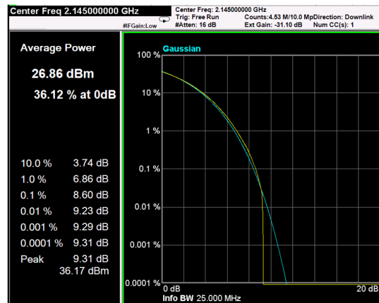
Channel: MIDDLE, Modulation: 256QAM, BW=20MHz, CCDF
