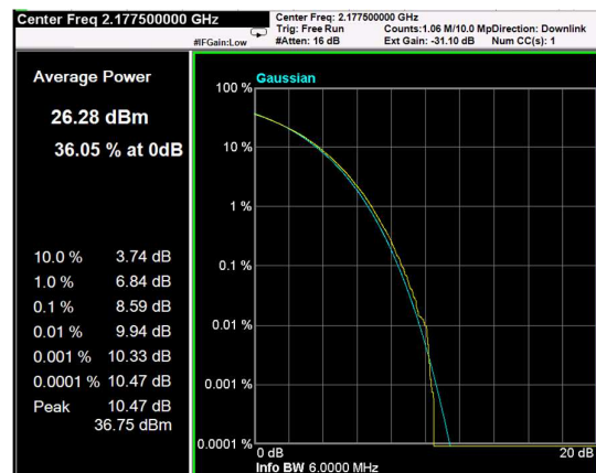
Channel: TOP, Modulation: 16QAM, BW=5MHz, CCDF
