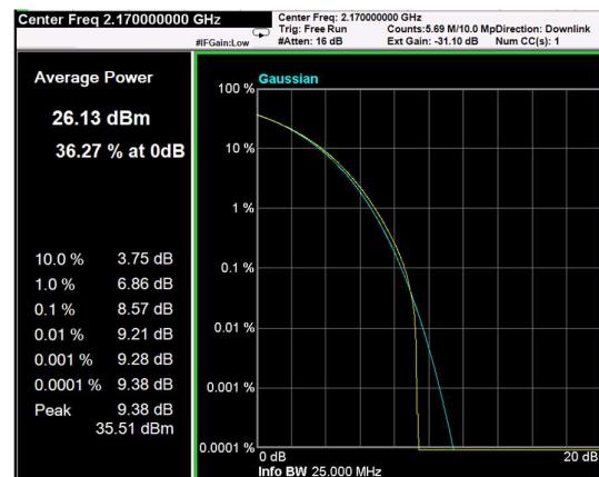
Channel: TOP, Modulation: 16QAM, BW=20MHz, CCDF
