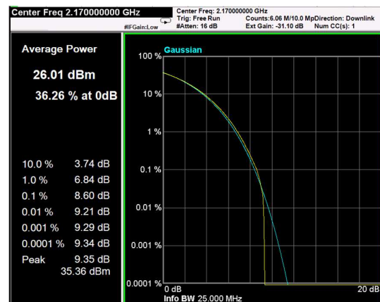
Channel: TOP, Modulation: 64QAM, BW=20MHz, CCDF
