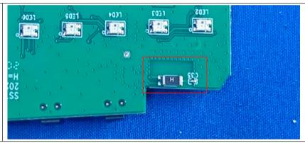
The antenna is Chip antenna.
