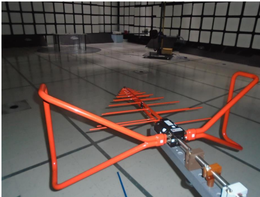
Photograph 6. Radiated Emissions, 30 – 1000 MHz, Antenna
