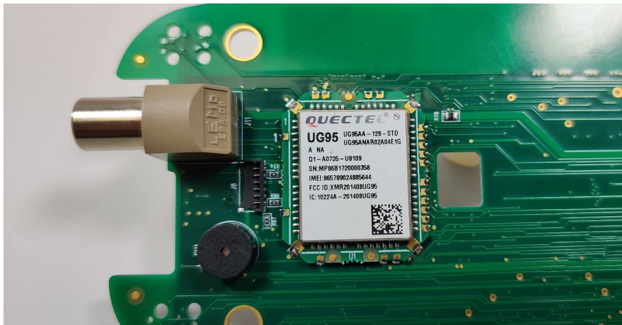
Internal Picture 5: Quectel UG95 3G modem that is firmware disabled in the Vesta Charger systems, but is populated.
