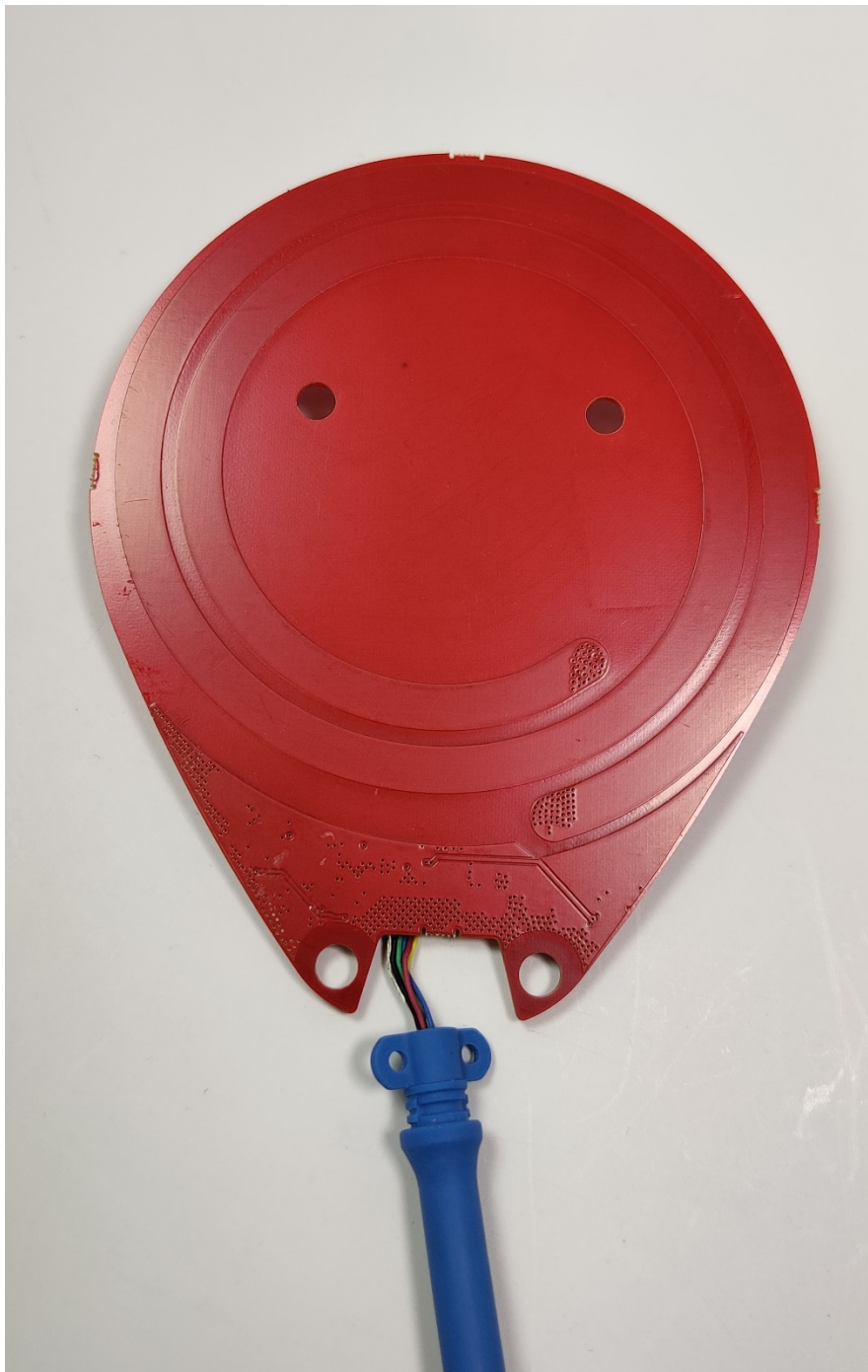
Internal Picture 8: Bottom PCB layout for charging coil board. A 2-turn PCB trace antenna encompasses the majority of the bottom layout and is used for the 13.56MHz wireless power transfer coil.
