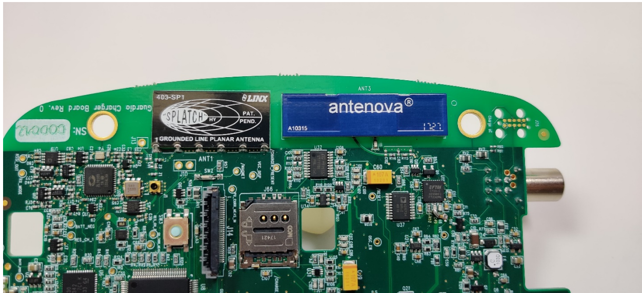
Internal Picture 3: Antennas present on the main board. 403MHz MICs antenna is Linx Technologies ANT-403-SP (left, black). GSM/UMTS antenna is Antennova A10315 that is disabled in Vesta Charger systems (right, blue).
