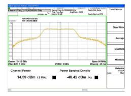
802.11g, 6 and 54 Mbps Mid Channel = 2437 MHz Output Power @ 6 Mbps = 15.59 dBm Output Power @ 54 Mbps = 15.53 dBm
