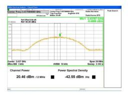
802.11b, 1 and 11 Mbps High Channel = 2462 MHz PSD @ 1 Mbps = -8.0483 dBm PSD @ 11 Mbps = -6.8998 dBm
