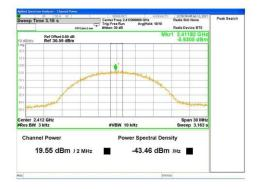
802.11b, 1 and 11 Mbps Mid Channel = 2437 MHz PSD @ 1 Mbps = -4.76 dBm PSD @ 11 Mbps = -5.48 dBm
