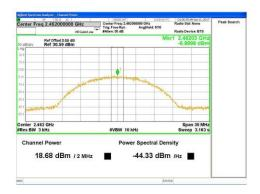
802.11g, 6 and 54 Mbps Low Channel = 2412 MHz PSD @ 1 Mbps = -9.767 dBm PSD @ 11 Mbps = -9.389 dBm
