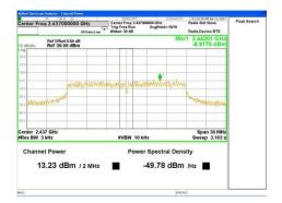
802.11n, 20 MHz BW, MCS0 and MCS7 High Channel = 2462 MHz PSD @ MCS0 = -9.3823 dBm PSD @ MCS7 = -11.662 dBm
