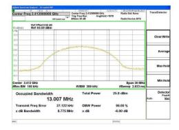
802.11b, 1 and 11 Mbps Mid Channel = 2437 MHz 6dB BW @ 1 Mbps = 9.084 MHz 6dB BW @ 11 Mbps = 8.952 MHz
