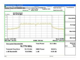
802.11g, 6 and 54 Mbps High Channel = 2462 MHz 6dB BW @ 1 Mbps = 16.38 MHz 6dB BW @ 11 Mbps = 16.46 MHz
