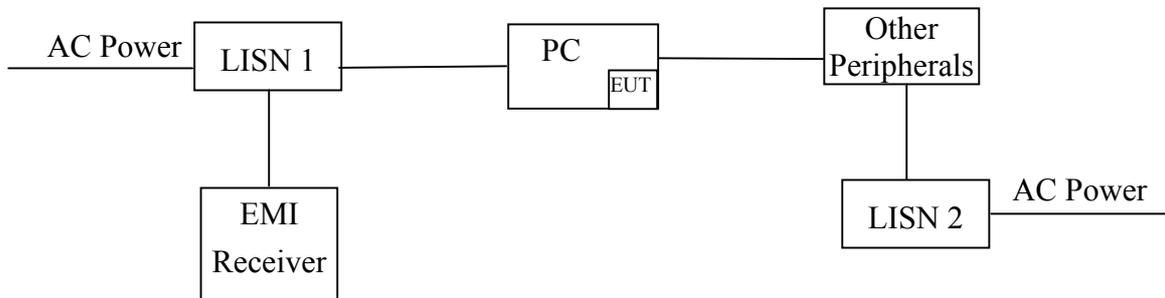
The EUT are connected to the main power through a line impedance stabilization network (LISN). This provides a 50 ohm/50uH coupling impedance for the measuring equipment. The peripheral devices are also connected to the main power through a LISN that provides a 50ohm/50uH coupling impedance with 50ohm termination.
