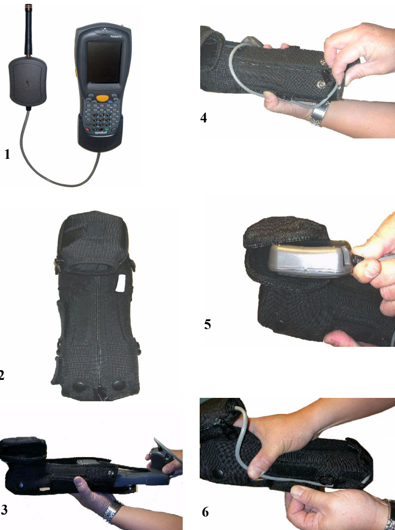
Figure 3-1 Connecting the SMR-650P-211 Reader
