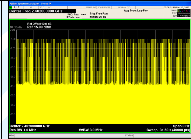
Number of Pulses in 31.6 seconds 8DPSK_3-DH3
