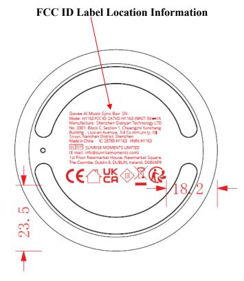
The label shown shall be permanently affixed at a conspicuous location on the device and be readily visible to the user at the time purchase (Labeling requirements per 2.925)
