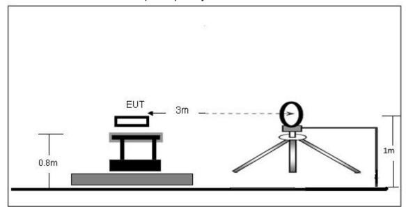
(B) Radiated Emission Test-Up Frequency 30MHz~1GHz
