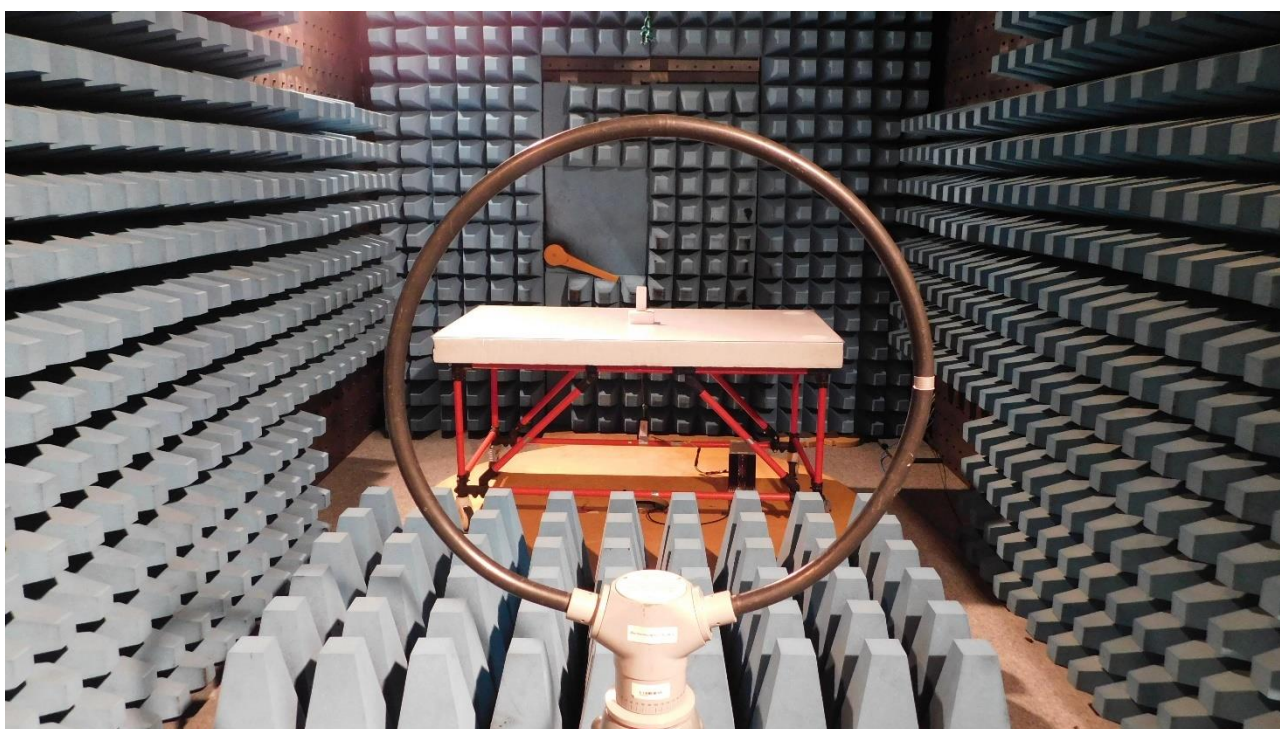
Picture 2: CDC, test setup radiated emission test 9 kHz - 30 MHz (rear view)
