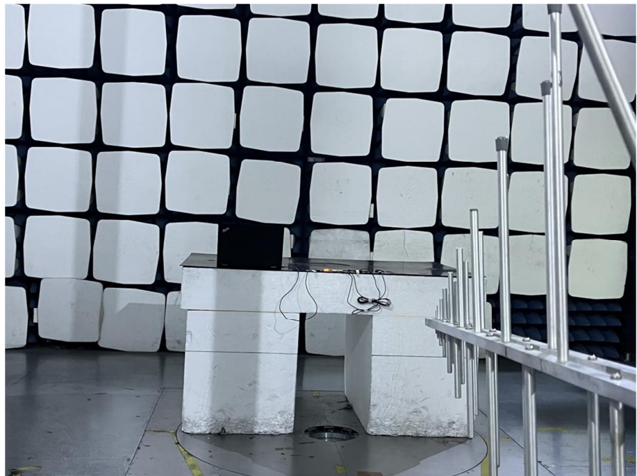
Radiation Emission Test Setup (30MHz to 1GHz)
