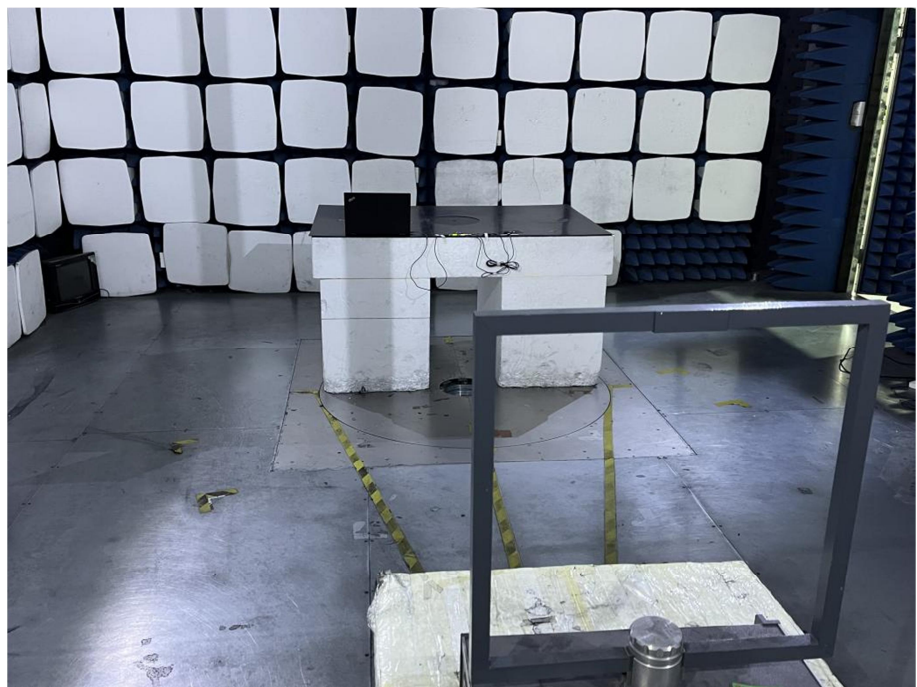
Radiation Emission Test Setup (Below 30MHz)
