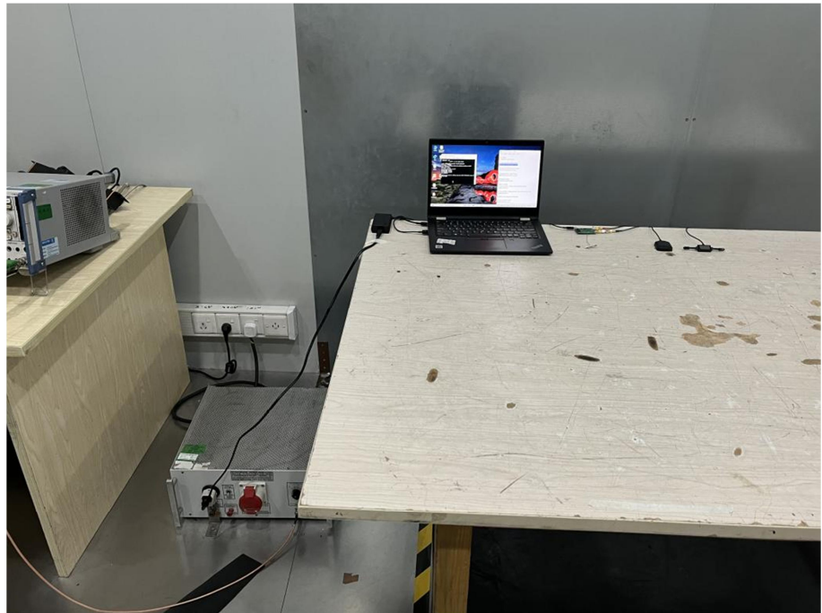
Conducted Emission Test Setup
