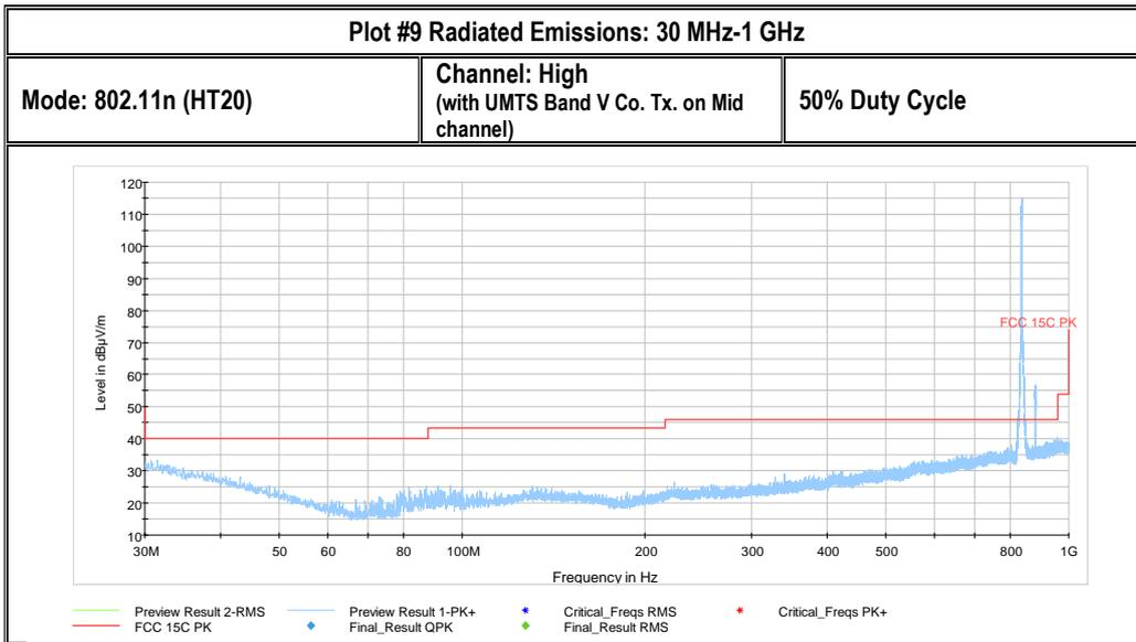
Note: Intentional Transmission occurring on UMTS Band V: 836.5 MHz (uplink), 881.5 MHz (downlink) exceeding the FCC 15.247 test limit is acceptable due to UMTS Band V being regulated by FCC part 22 limits therefore not subjected to FCC 15.247 regulations.
