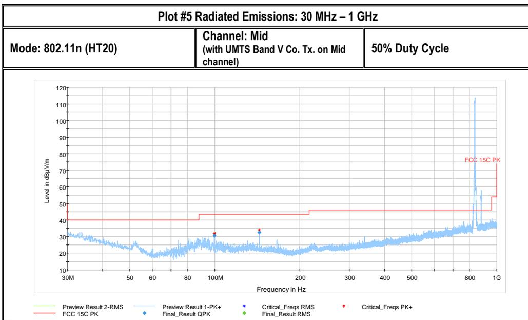
Note: Intentional Transmission occurring on UMTS Band V: 836.5 MHz (uplink), 881.5 MHz (downlink) exceeding the FCC 15.247 test limit is acceptable due to UMTS Band V being regulated by FCC part 22 limits therefore not subjected to FCC 15.247 regulations.
