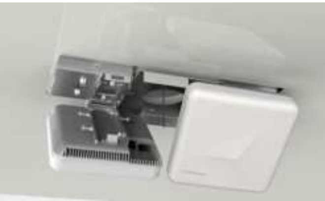
Figure 72. Buckle the Bracket 2
