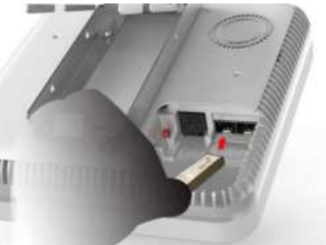
Figure 73. SFP Module Insertion
