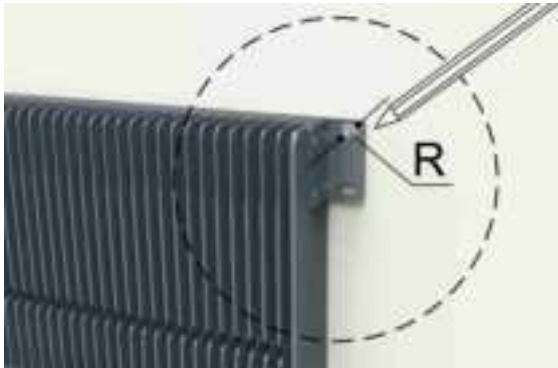
Figure 31. Marking the Position of Mounting Holes
