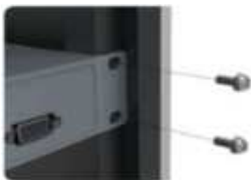
Figure 26. Fix EU-O with Screws
