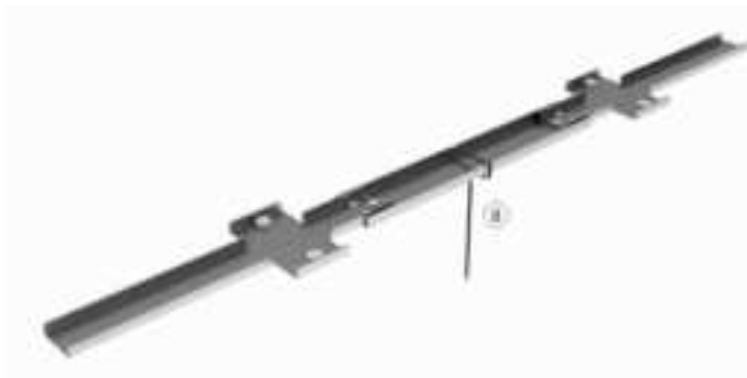
Figure 62. Attaching Cable Tie to Mounting Bracket
