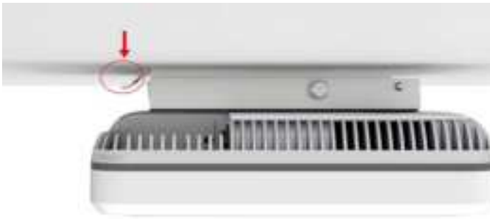
Figure 46. Unlock Rotary Hook Diagram 1
