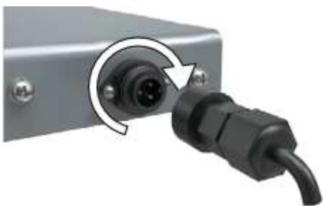
Figure 28. Connect Power Cable at Rear Side
