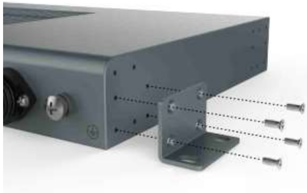
Figure 30. Attaching a 19-in Mounting Bracket
