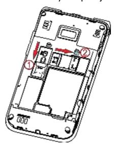
Step 4. Re-install the battery by aligning the gold contact points of the battery with the gold contact points of the cave. It only fits one way. Press down to snap in place.
