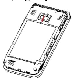
Step 3. To insert SIM card or microSD card, push the SIM card or microSD card into the card slot with the gold-colored contacts facing down.
