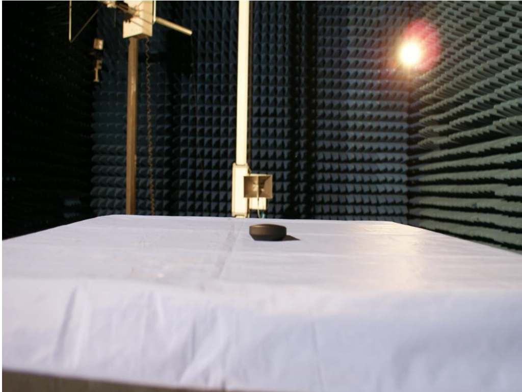
Photograph 4: Set-up for Spurious Emissions (18GHz-26GHz)
