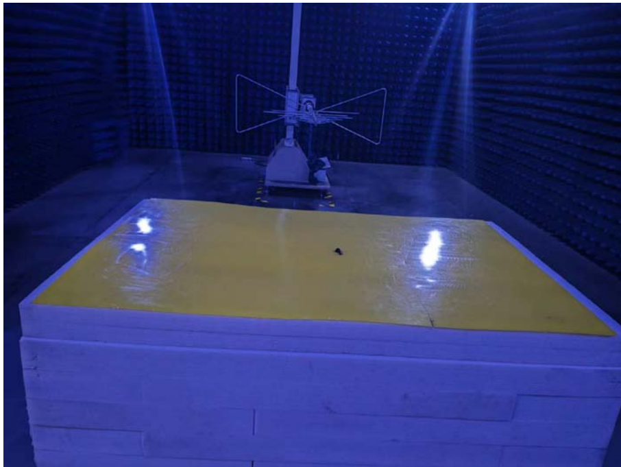
Photo of Radiated Emission Measurement Below 1GHz
