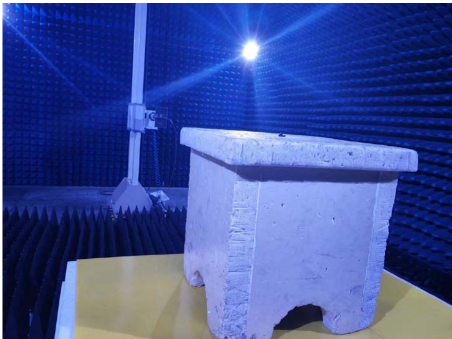
Photo of Radiated Emission Measurement Above 1GHz
