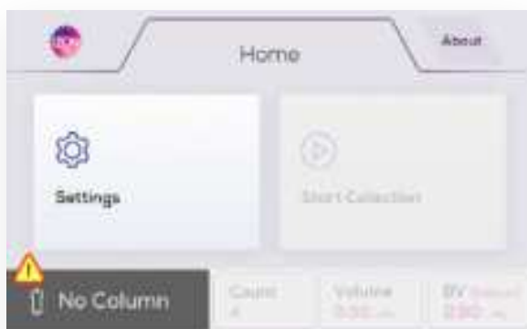
Figure 8: Home screen when no column is attached to the AFC.
