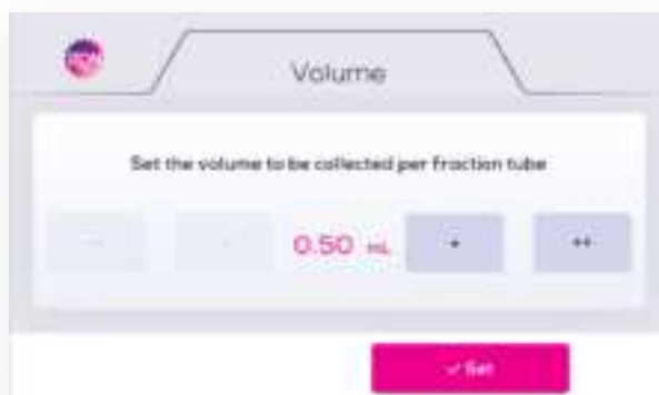
Figure 16: The Volume screen allows you to adjust the volume to be collected per fraction. Press -/+ to adjust in small increments or --/++ to adjust in large increments. Press Set to save your parameters and return to the home screen.
