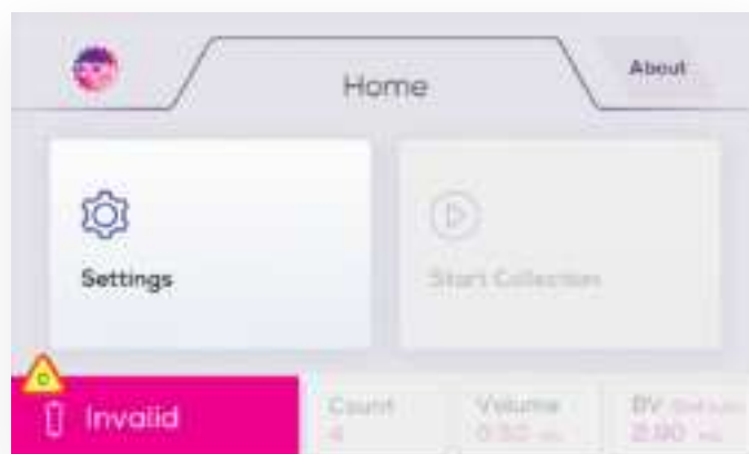
Figure 13: The home screen displaying when a column is invalid.
