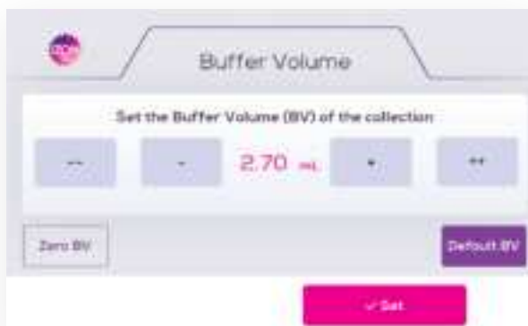
Figure 17: The Buffer Volume menu allows you to set the buffer volume of the collection run. Default BV sets the volume to the recommended buffer volume, while Zero BV sets the buffer volume to zero. Press -/+ to adjust in small increments and --/++ to adjust in large increments. Press Set to save your parameters and return to the home screen.
