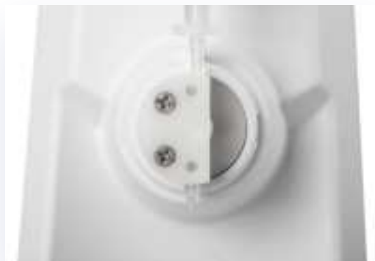
Figure 24: Pinch valve cover removed; pull tube laterally.
