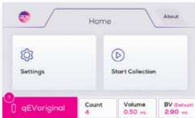
Figure 11: A circle indicator shows how many recommended uses a column has left.
