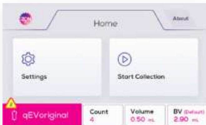
Figure 12: A warning indicator shows how many uses a column has left after the recommended uses have been exceeded.
