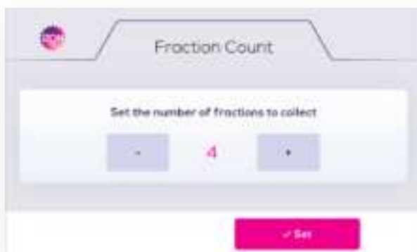
Figure 15: From the Count screen, you can adjust the fraction number. Press -/+ to choose your collection count. Press Set to save your parameters and return to the home screen.
