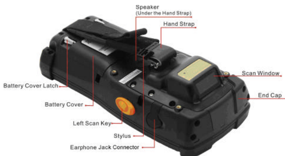
Figure 2-4 PHL-7100 rear view
