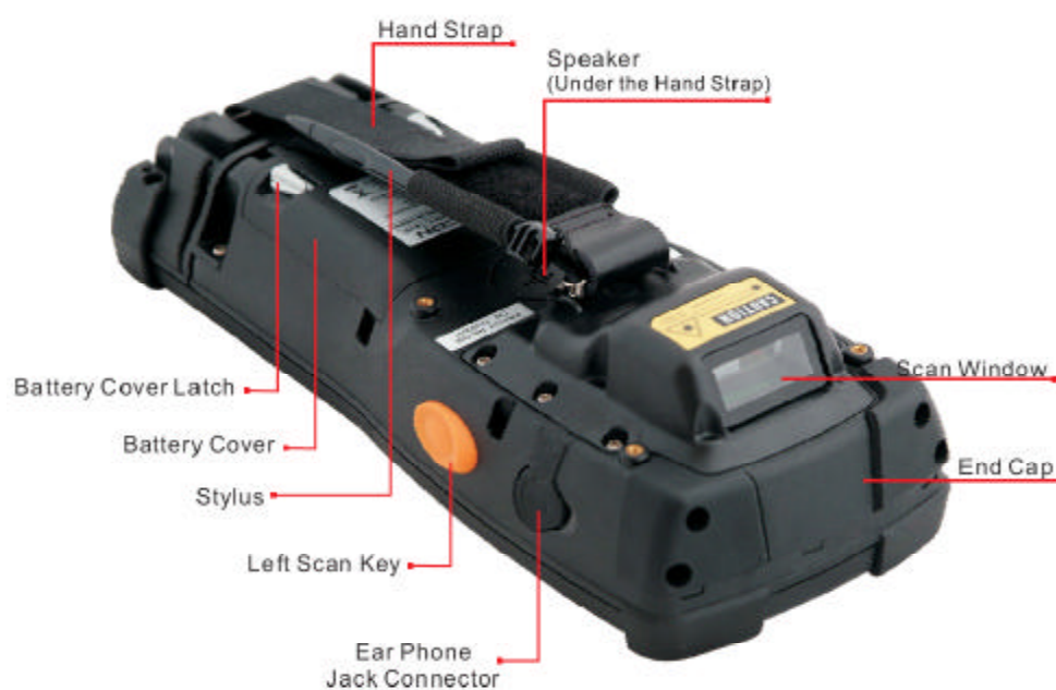
Figure 2-6 PHL-7200 rear view
