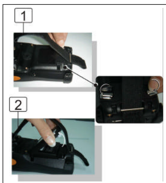
Figure 2-8 Detach the battery cover from PDT
