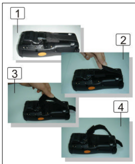
Figure 2-7 Release the Hand strap from PDT
