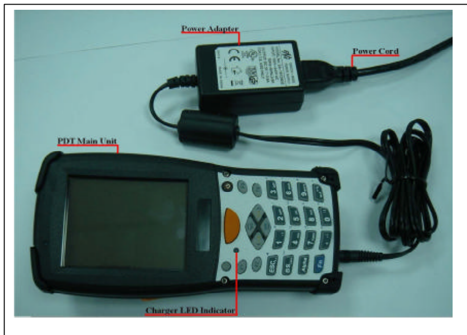
Figure 2-11 Charging with power adapter (PHL-7100 shown)
