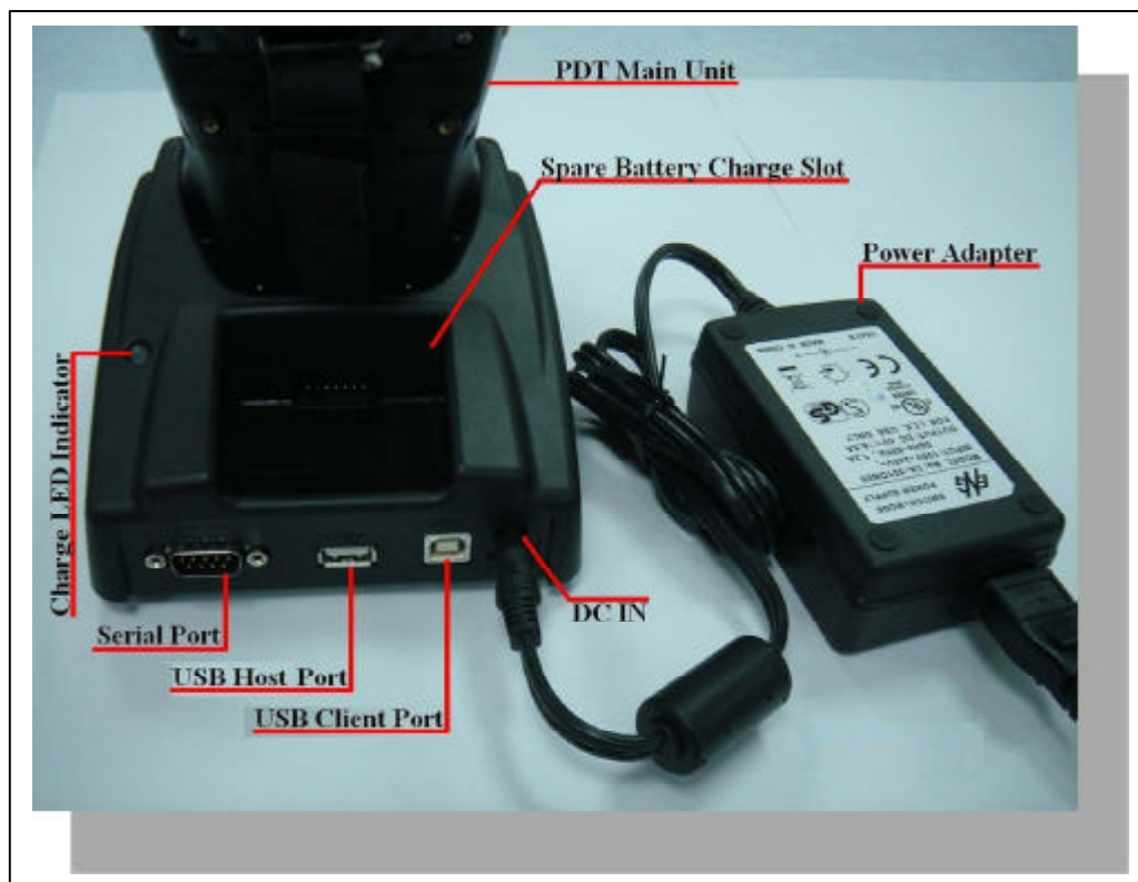
Figure 2-12 Charging with IRU-7000 cradle
