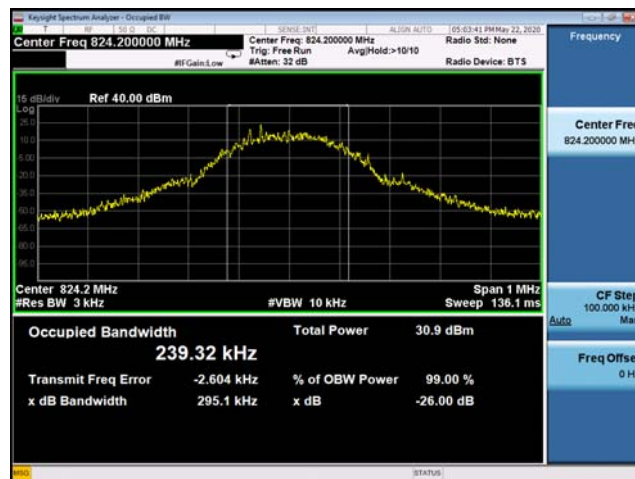
(Plot C1: EDGE 850MHz Channel = 128 Occupied bandwidth)
