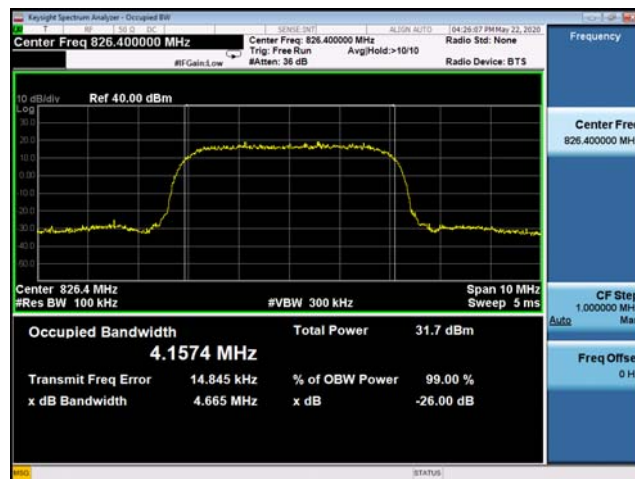
(Plot E1: WCDMA 850MHz Channel = 4132 Occupied bandwidth)
