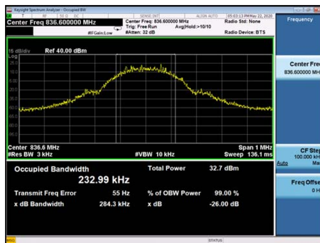
(Plot C2: EDGE 850MHz Channel = 190 Occupied bandwidth)
