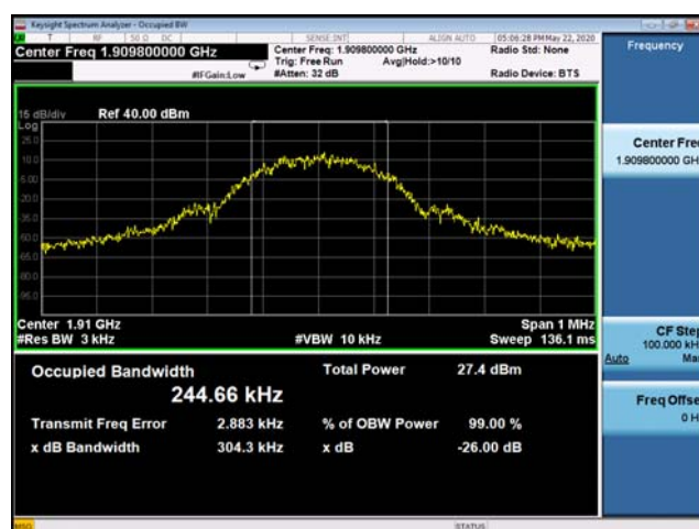
(Plot D3: EDGE 1900MHz Channel = 810 Occupied bandwidth)
