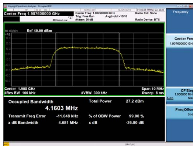
(Plot F3: WCDMA 1900MHz Channel = 9538 Occupied bandwidth)
