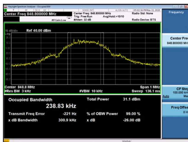
(Plot C3: EDGE 850MHz Channel = 251 Occupied bandwidth)
