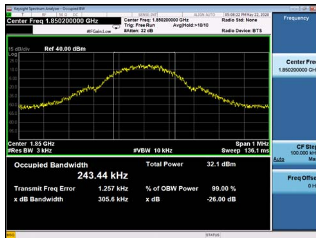
(Plot B1: GSM 1900MHz Channel = 512 Occupied bandwidth)
