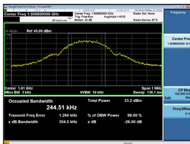
(Plot B3: GSM 1900MHz Channel = 810 Occupied bandwidth)
