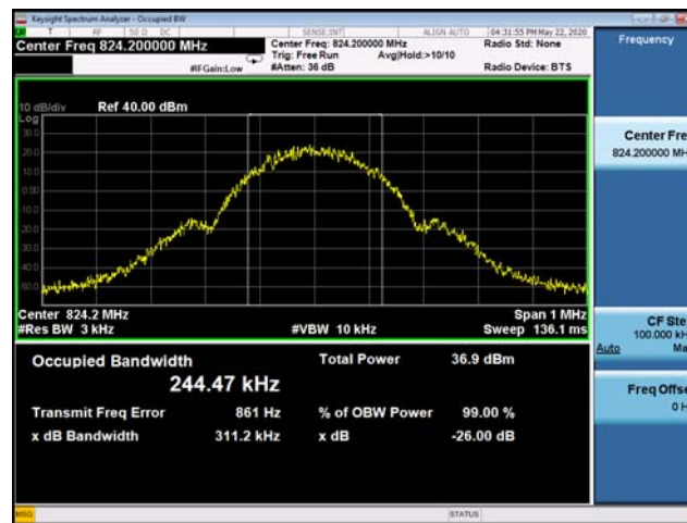
(Plot A1: GSM 850MHz Channel = 128 Occupied bandwidth)
