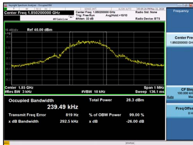
(Plot D1: EDGE 1900MHz Channel = 512 Occupied bandwidth)
