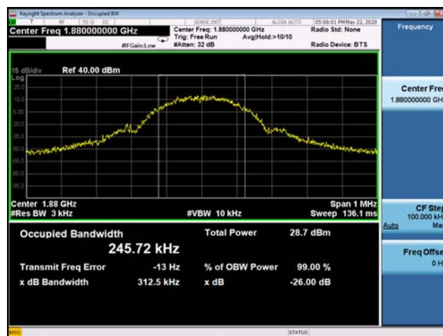
(Plot D2: EDGE 1900MHz Channel = 661 Occupied bandwidth)
