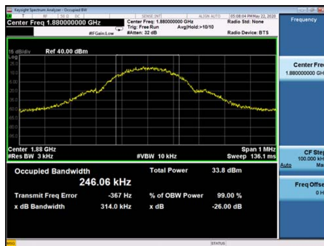
(Plot B2: GSM 1900MHz Channel = 661 Occupied bandwidth)
