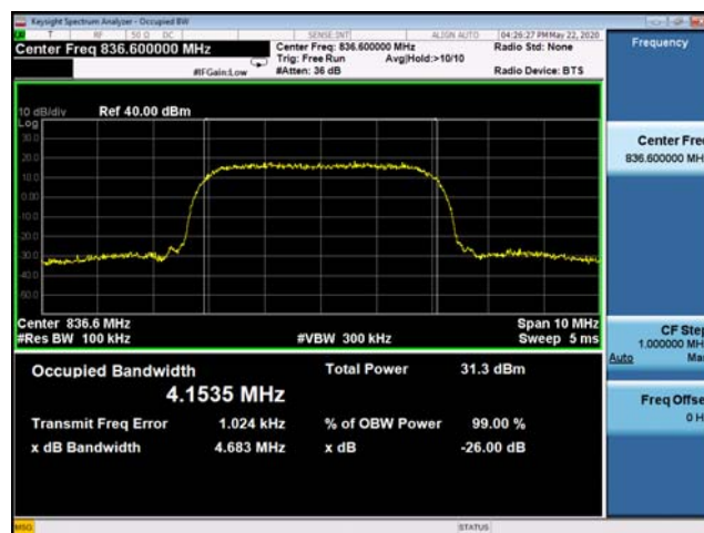
(Plot E2: WCDMA 850MHz Channel = 4183 Occupied bandwidth)
