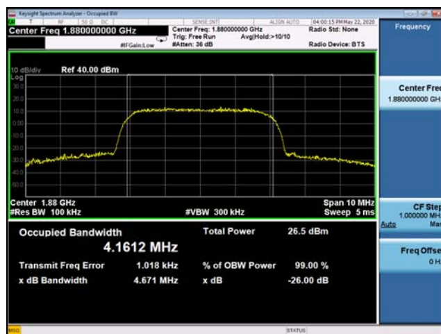
(Plot F2: WCDMA 1900MHz Channel = 9400 Occupied bandwidth)
