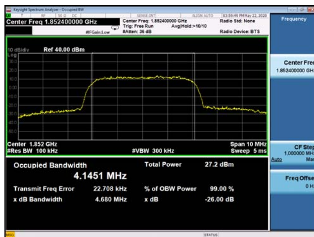
(Plot F1: WCDMA 1900MHz Channel = 9262 Occupied bandwidth)
