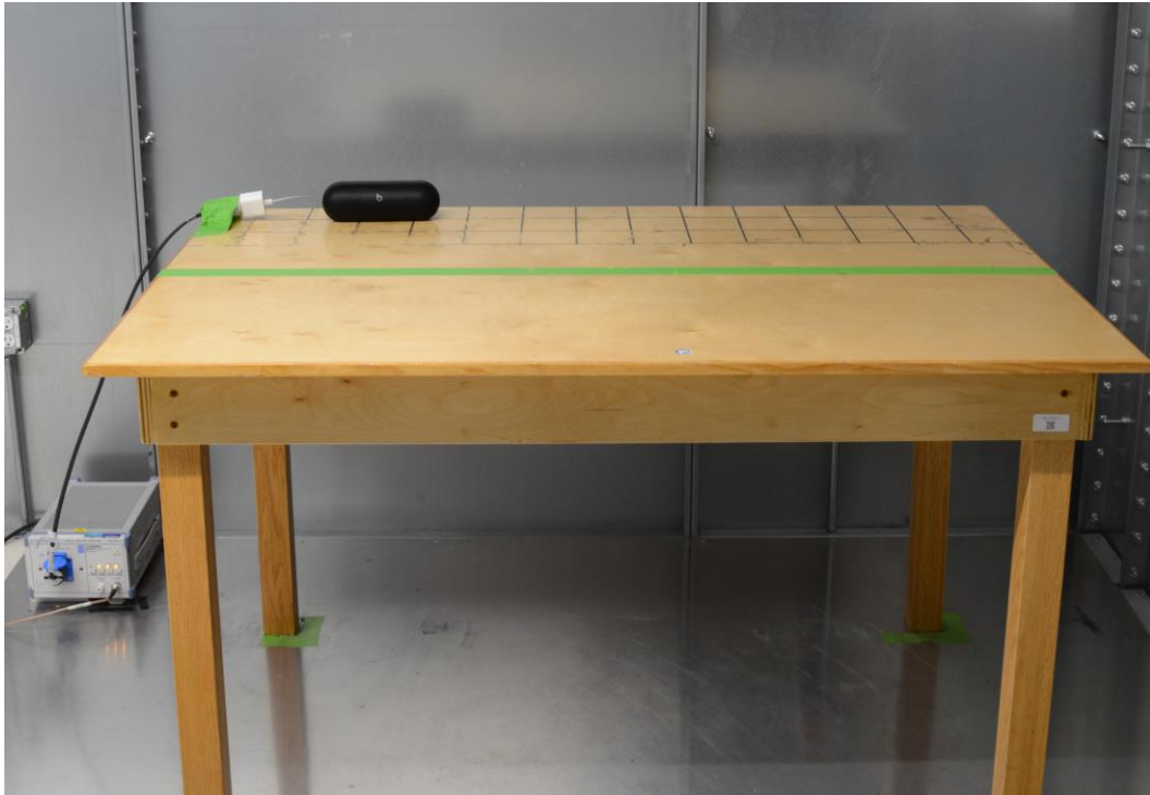
Figure 1: AC Line Conducted Emissions (Front View)
