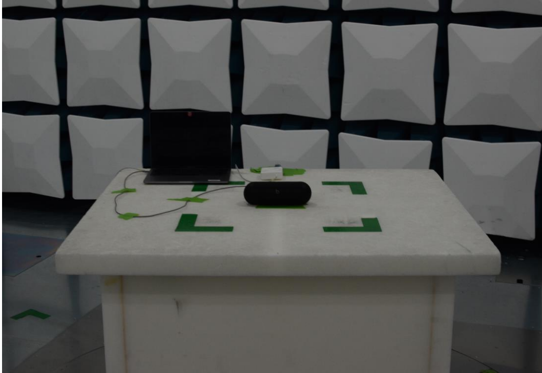
Figure 17: 30MHz-1GHz Test Setup (Front View)
