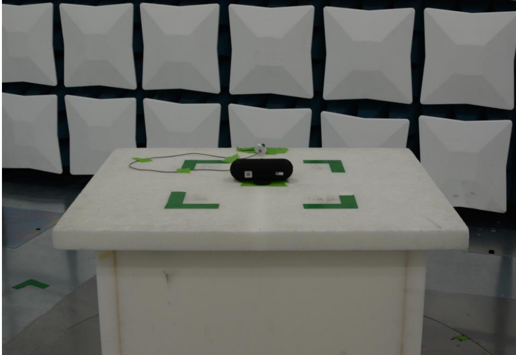
Figure 13: 30MHz-1GHz Test Setup (Front View)
