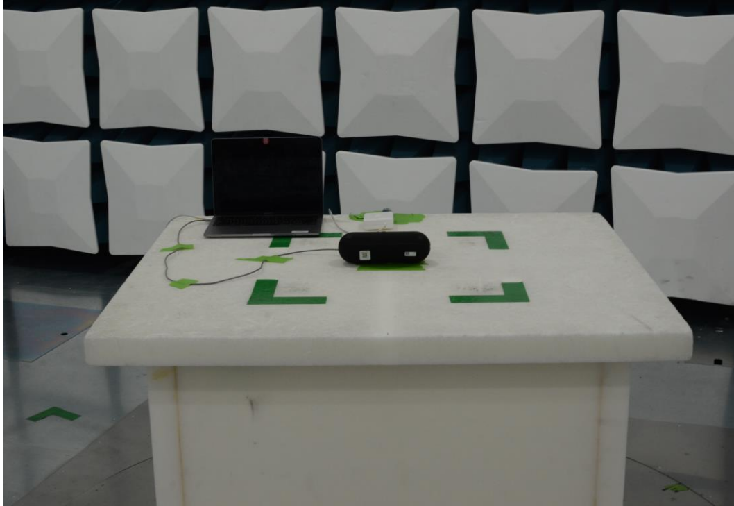
Figure 19: 30MHz-1GHz Test Setup (Front View)
