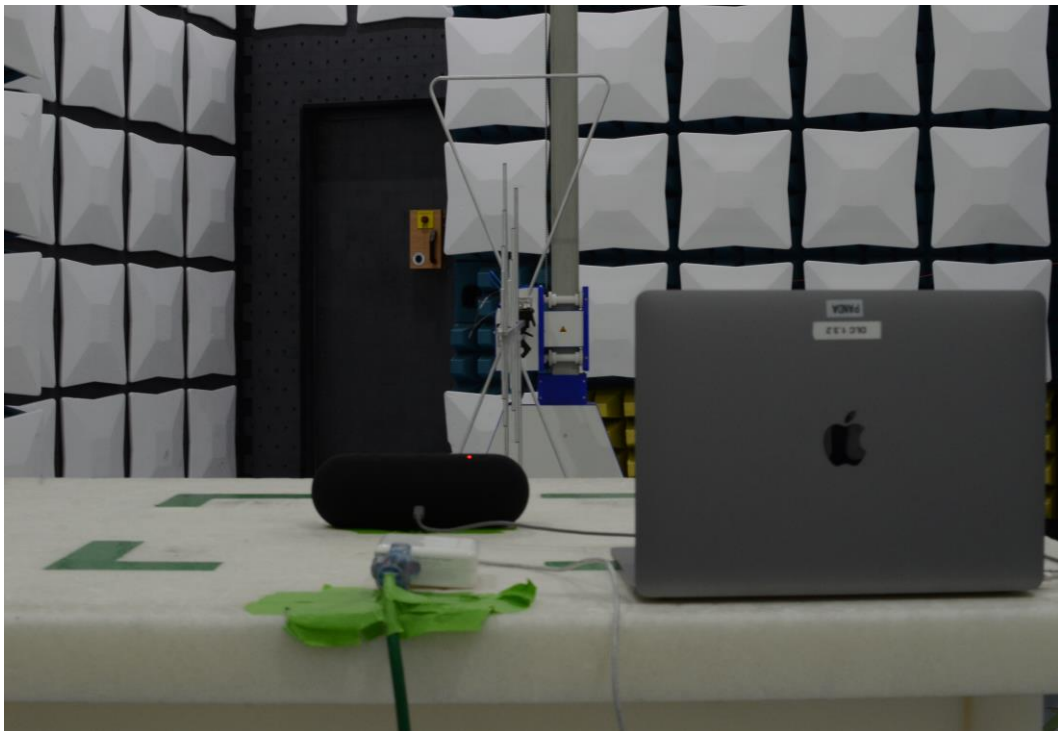
Figure 18: 30MHz-1GHz Test Setup (Rear View)
