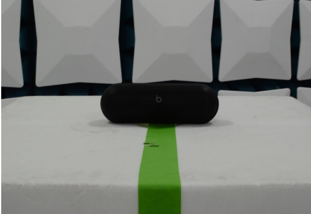
Figure 5: 1-18GHz Test Setup (Front View)
