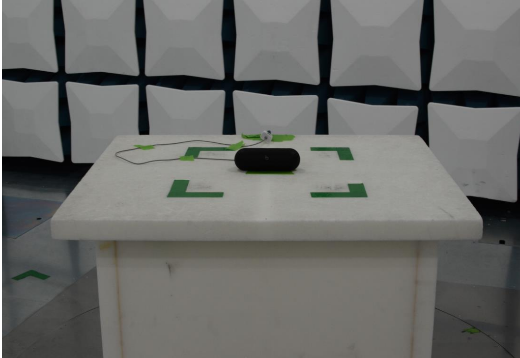
Figure 11: 30MHz-1GHz Test Setup (Front View)
