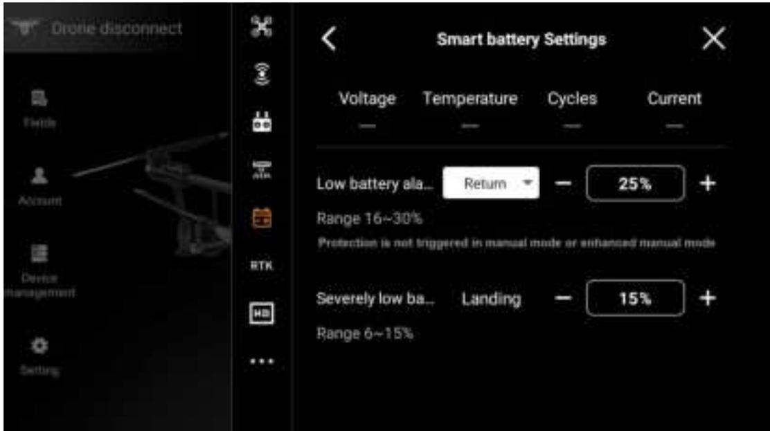
Note: The specific percentage of remaining power of low power can be set in the agricultural UAV APP. It is recommended that users set it relatively conservatively to ensure flight safety
