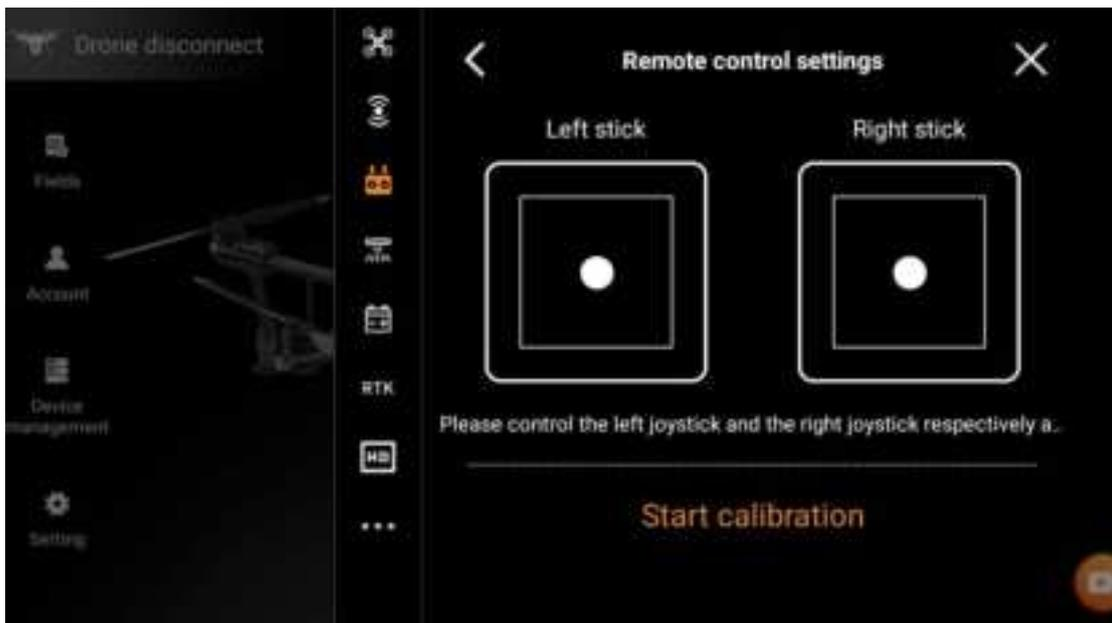
Click "Calibration" to enter the joystick calibration interface, and click "Start Calibration"
