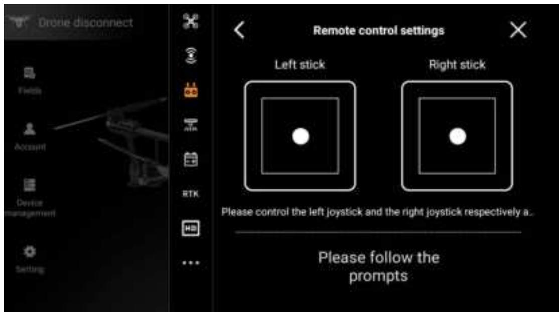
After filling in the square ring shape, the joystick calibration can be completed.
