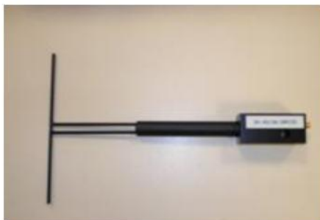
Figure 1 – Satimo COMOSAR Validation Dipole
