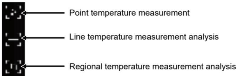
(1) Point temperature measurement: click the point temperature measurement button, and the screen will display the temperature information of three points, namely the central temperature point, the highest temperature point and the lowest temperature point. Click the screen at this time, and the temperature information of the user-defined point will be added.
