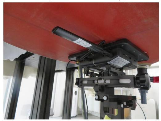
Description: Right 30° antenna position for screen side with 0mm gap
