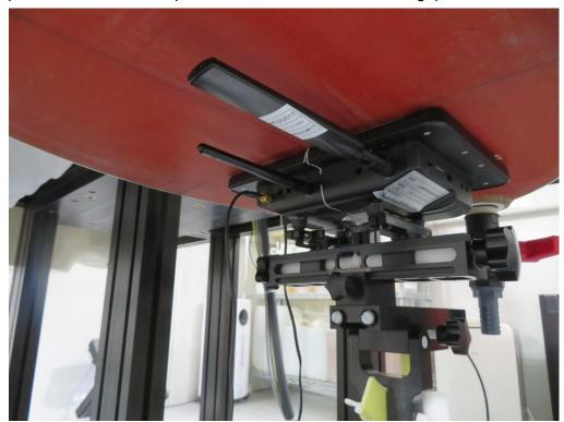
Description: Front 30° antenna position for screen side with 0mm gap
