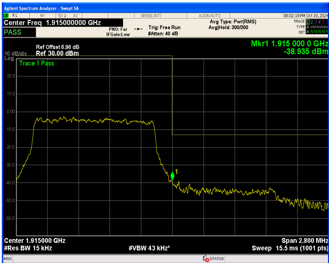
Band26a QPSK BW=1.4MHz Channel=26697 RB Size=1 Position=#0
