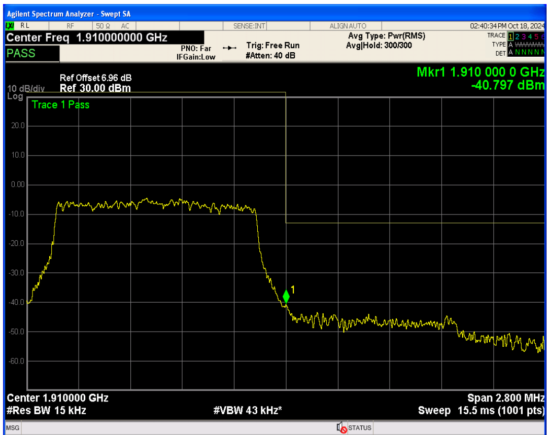
Band25 QPSK BW=1.4MHz Channel=26047 RB Size=1 Position=#0
