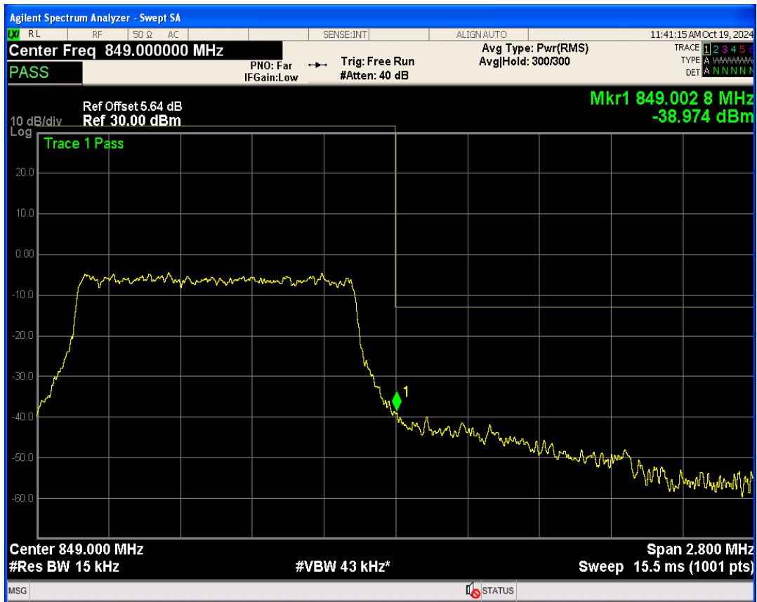
Band4 QPSK BW=1.4MHz Channel=19957 RB Size=1 Position=#0
