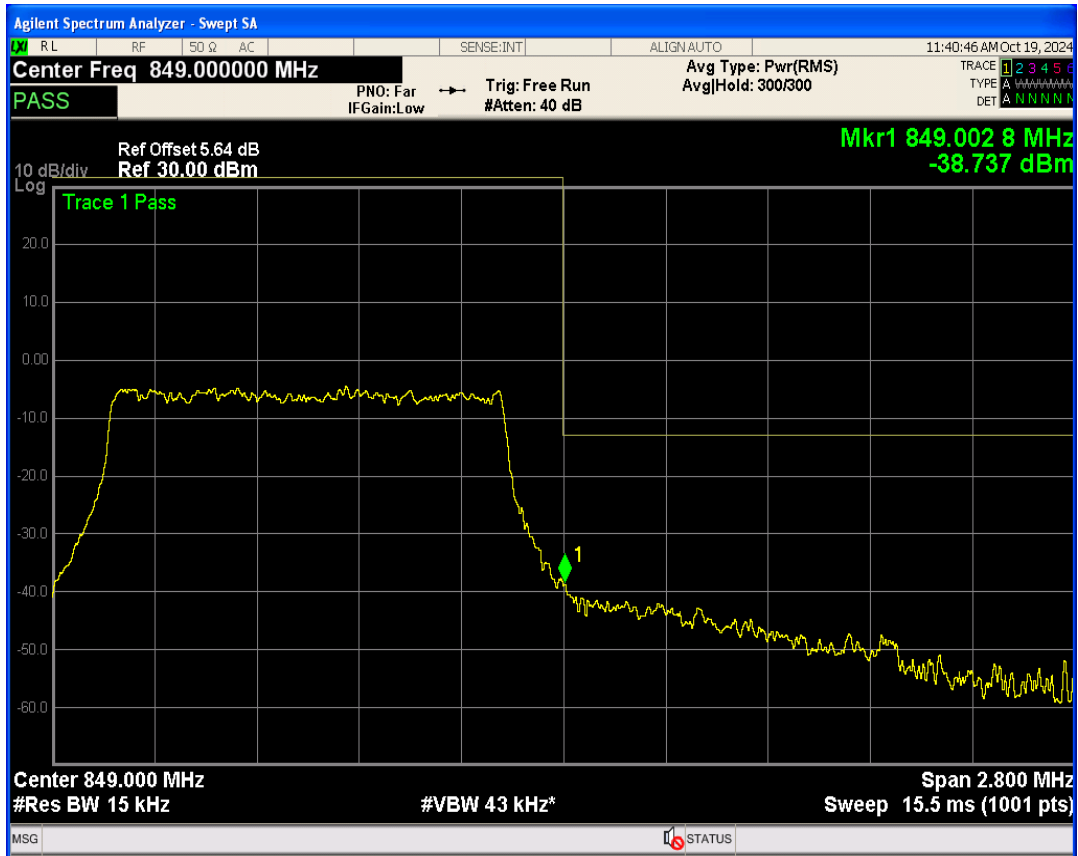
Band26b 16QAM BW=1.4MHz Channel=27033 RB Size=1 Position=#0
