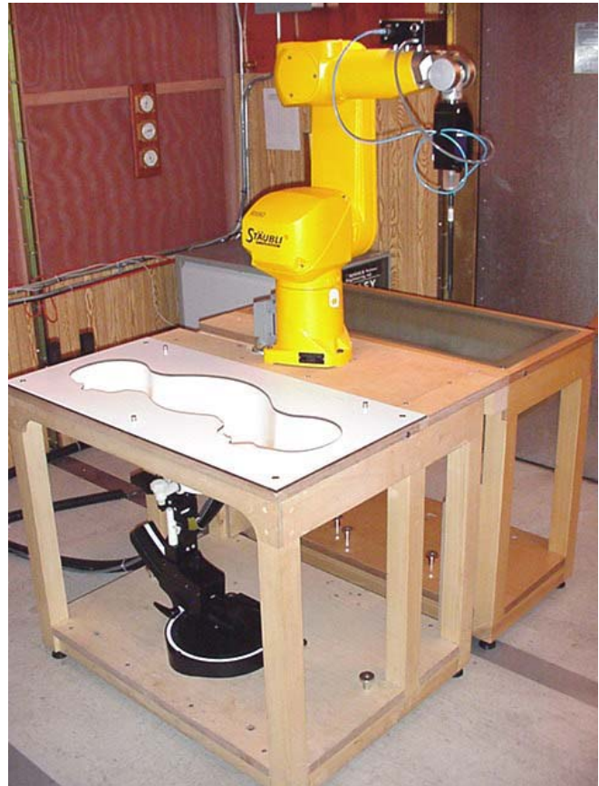
DASY4 SAR Measurement System with SAM phantom
