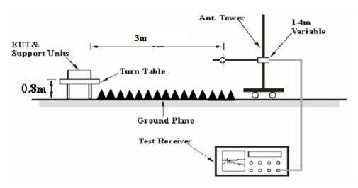
The radiated emission below 1GHz tests were performed in the 10 meters chamber test site, above 1GHz tests were performed in the 3 meters chamber test site A, using the setup accordance with the ANSI C63.4-2014. The specification used was with the FCC Part 15 B Class B limits.
