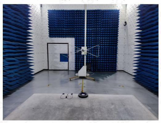
RADIATED EMISSION TEST SETUP ABOVE 1GHz
