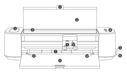
"B": Blade Clamp; "P": Pen Clamp Note: Please insert the blade or pen into the right clamp. Otherwise, the machine will be damaged.
