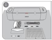
Take out the machine and the accessories from the package box and place them in a flat place. (Note: Please leave 12 inches (300mm) in front of and behind the machine for further operation.)
