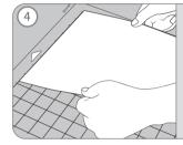
Pull off the clear film from your cutting mat and stick your material on the mat. (Note: Please make sure the cutting side of the material is facing up. Otherwise, the blade and the machine will get damaged.)
