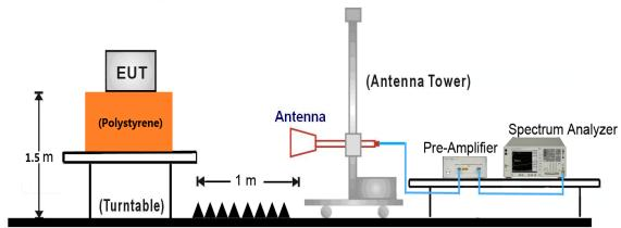
Note: This item was performed with the Bluetooth antenna connected.
