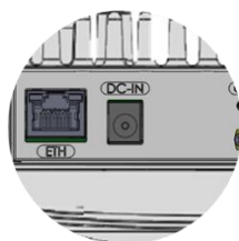
Figure 19: DC In - Panel
