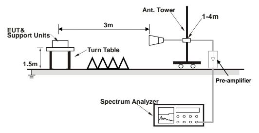
For radiated test above 18GHz
