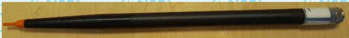
Figure 2 – MVG COMOSAR Dosimetric E field Dipole
