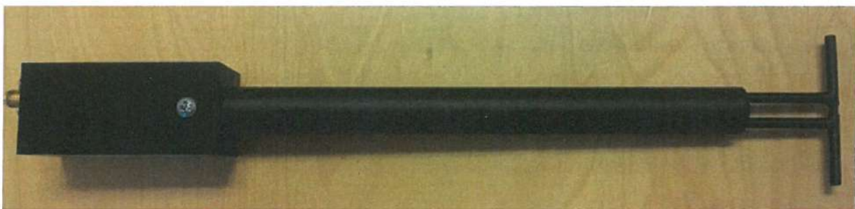
Figure 1 – MVG COMOSAR Validation Dipole
