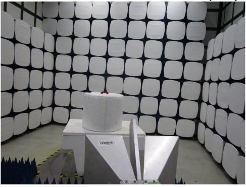
1.2 Radiated Emissions Test Setup
