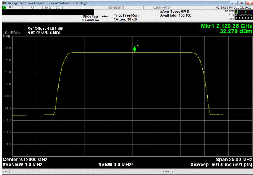
30 Watt Port 1, Band 1, 2110 MHz - 2155 MHz, 20 MHz Bandwidth, QPSK Modulation, Mid Channel 2132.5 MHz
