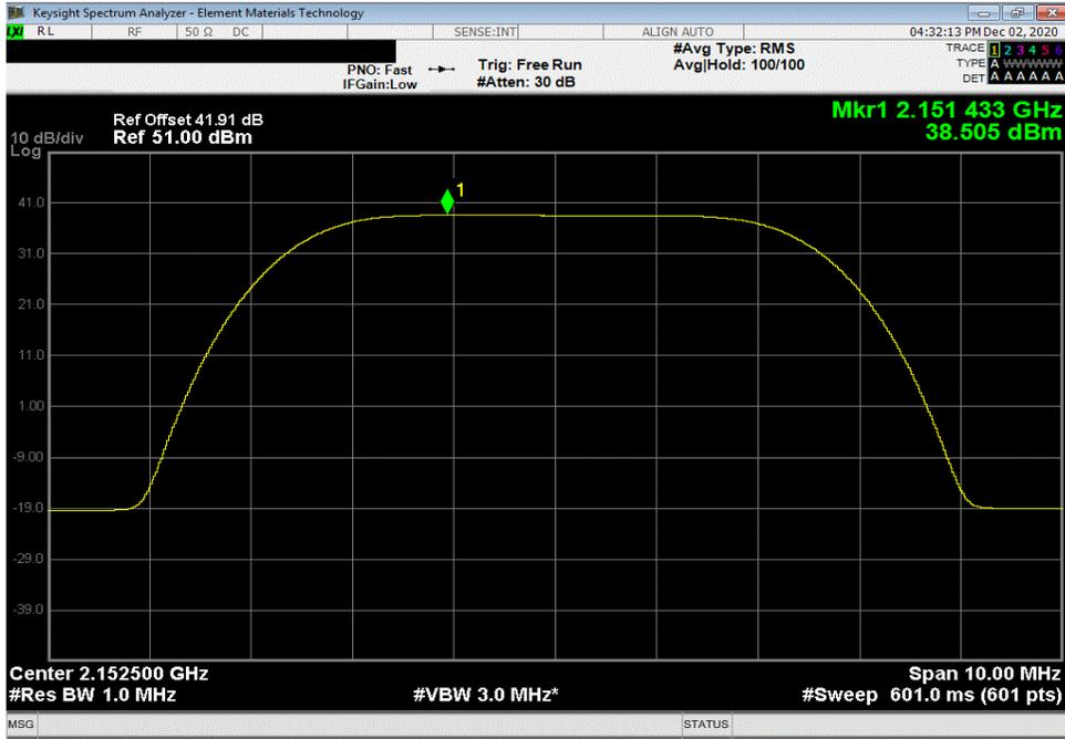
30 Watt Port 1, Band 1, 2110 MHz - 2155 MHz, 5 MHz Bandwidth, 256-QAM Modulation, Low Channel 2112.5 MHz
