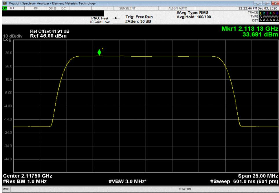
30 Watt Port 1, Band 1, 2110 MHz - 2155 MHz, 15 MHz Bandwidth, 64-QAM Modulation, Mid Channel 2132.5 MHz
