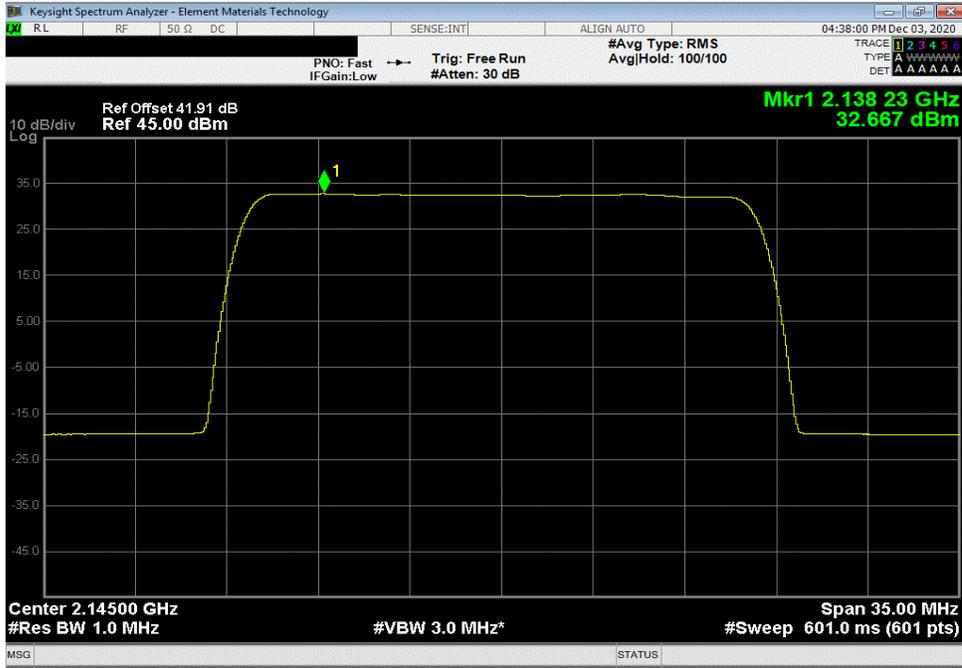
30 Watt Port 1, Band 1, 2110 MHz - 2155 MHz, 20 MHz Bandwidth, 256-QAM Modulation, Low Channel 2120 MHz
