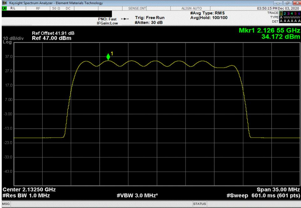
30 Watt Port 1, Band 1, 2110 MHz - 2155 MHz, 20 MHz Bandwidth, 16-QAM Modulation, High Channel 2145 MHz
