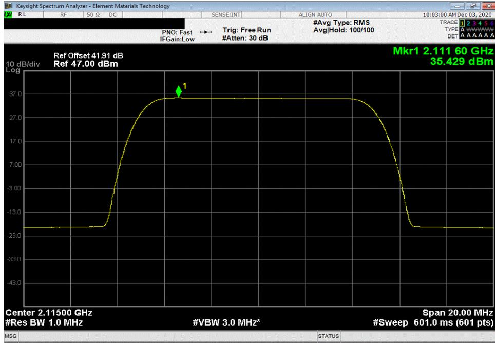
30 Watt Port 1, Band 1, 2110 MHz - 2155 MHz, 10 MHz Bandwidth, 64-QAM Modulation, Mid Channel 2132.5 MHz
