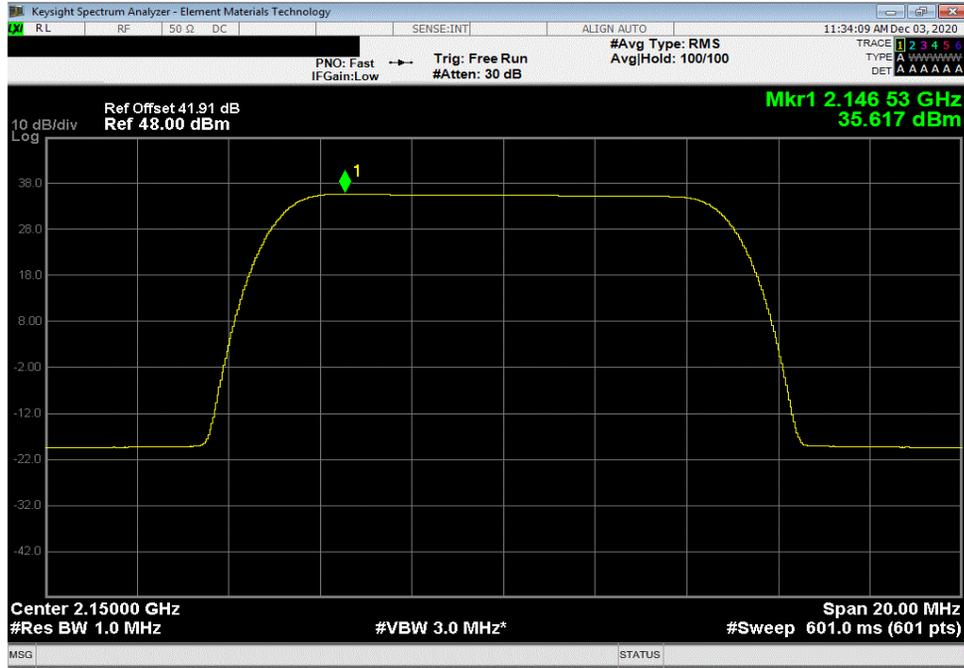
30 Watt Port 1, Band 1, 2110 MHz - 2155 MHz, 10 MHz Bandwidth, 256-QAM Modulation, Low Channel 2115 MHz
