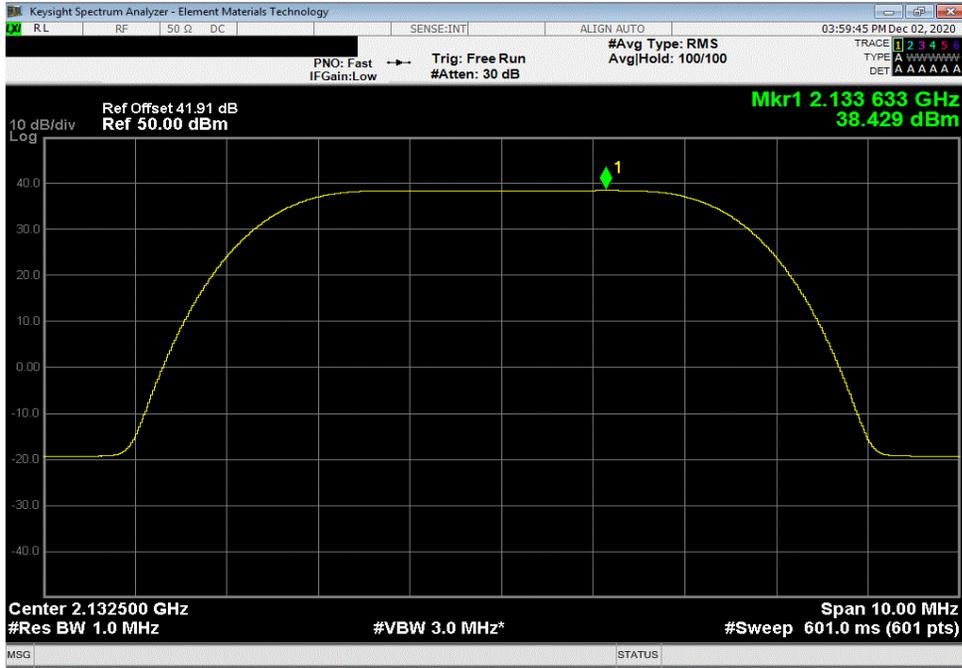
30 Watt Port 1, Band 1, 2110 MHz - 2155 MHz, 5 MHz Bandwidth, 256-QAM Modulation, High Channel 2152.5 MHz
