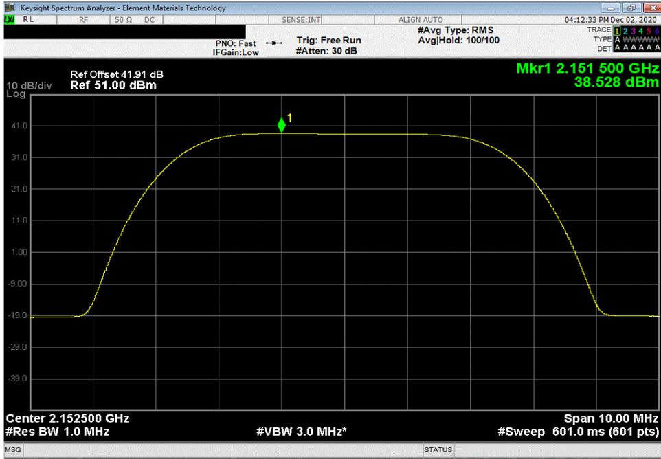
30 Watt Port 1, Band 1, 2110 MHz - 2155 MHz, 5 MHz Bandwidth, 16-QAM Modulation, Low Channel 2112.5 MHz
