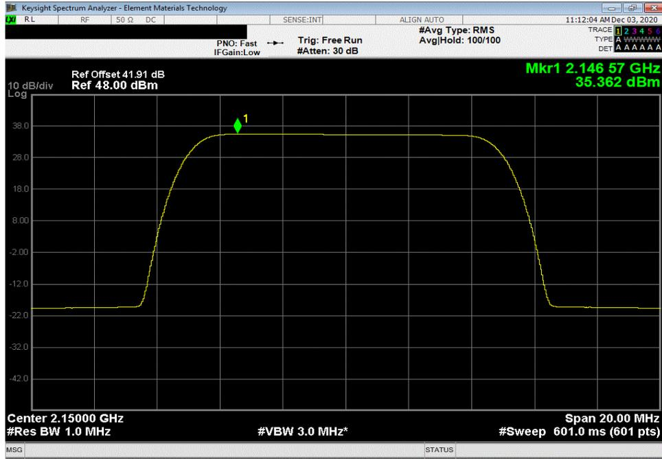
30 Watt Port 1, Band 1, 2110 MHz - 2155 MHz, 10 MHz Bandwidth, 16-QAM Modulation, Low Channel 2115 MHz
