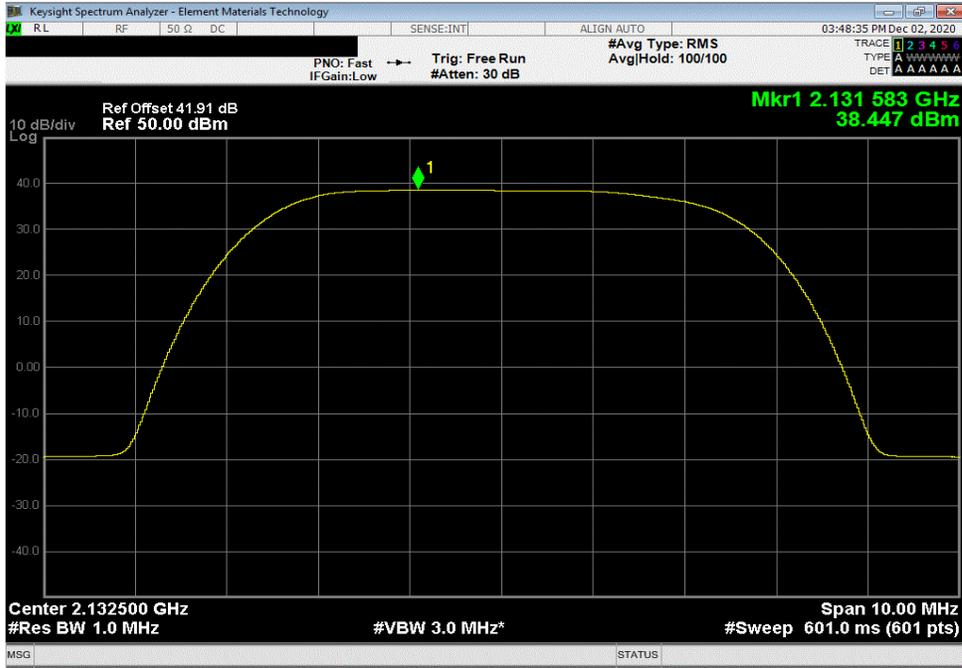
30 Watt Port 1, Band 1, 2110 MHz - 2155 MHz, 5 MHz Bandwidth, 16-QAM Modulation, High Channel 2152.5 MHz
