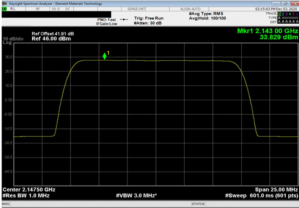
30 Watt Port 1, Band 1, 2110 MHz - 2155 MHz, 15 MHz Bandwidth, 256-QAM Modulation, Low Channel 2117.5 MHz
