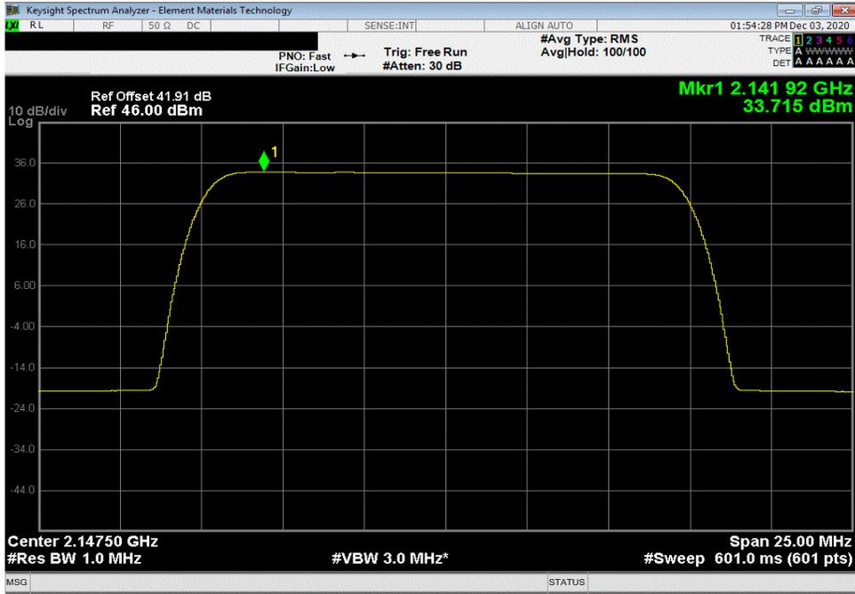
30 Watt Port 1, Band 1, 2110 MHz - 2155 MHz, 15 MHz Bandwidth, 16-QAM Modulation, Low Channel 2117.5 MHz
