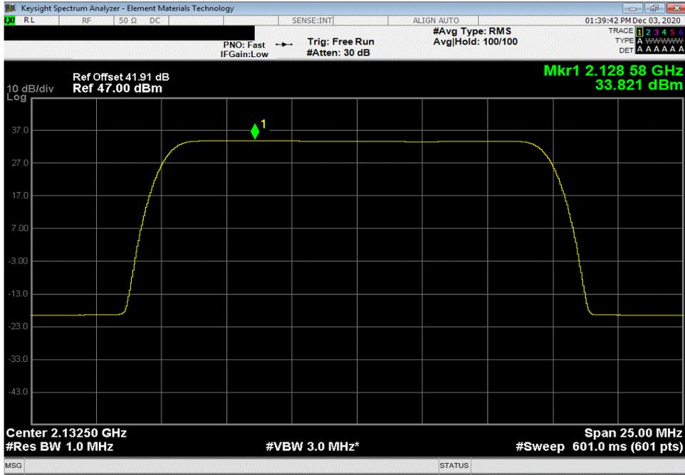
30 Watt Port 1, Band 1, 2110 MHz - 2155 MHz, 15 MHz Bandwidth, 256-QAM Modulation, High Channel 2147.5 MHz
