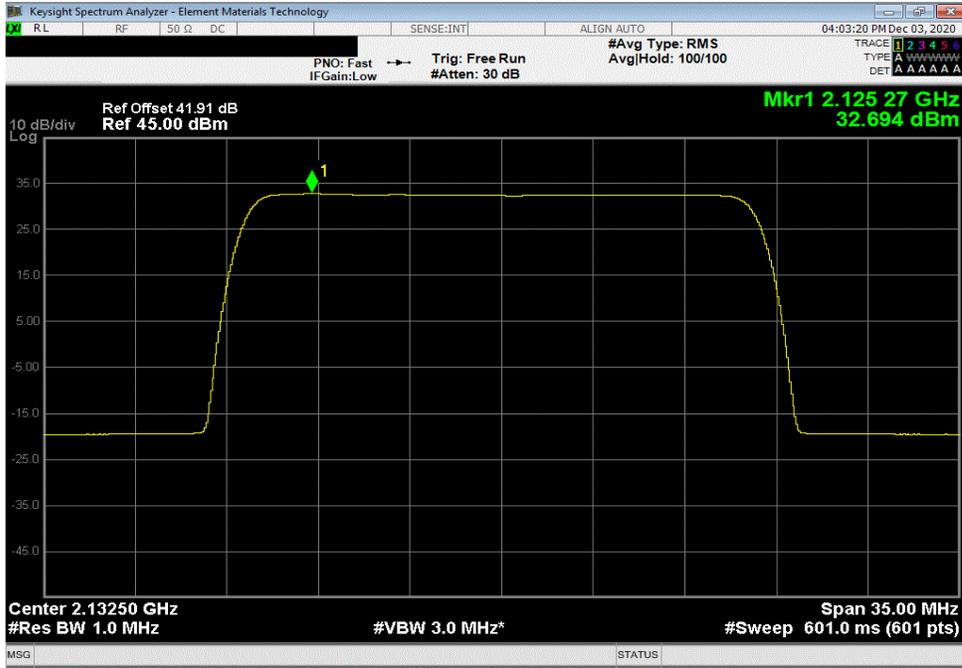
30 Watt Port 1, Band 1, 2110 MHz - 2155 MHz, 20 MHz Bandwidth, 256-QAM Modulation, High Channel 2145 MHz
