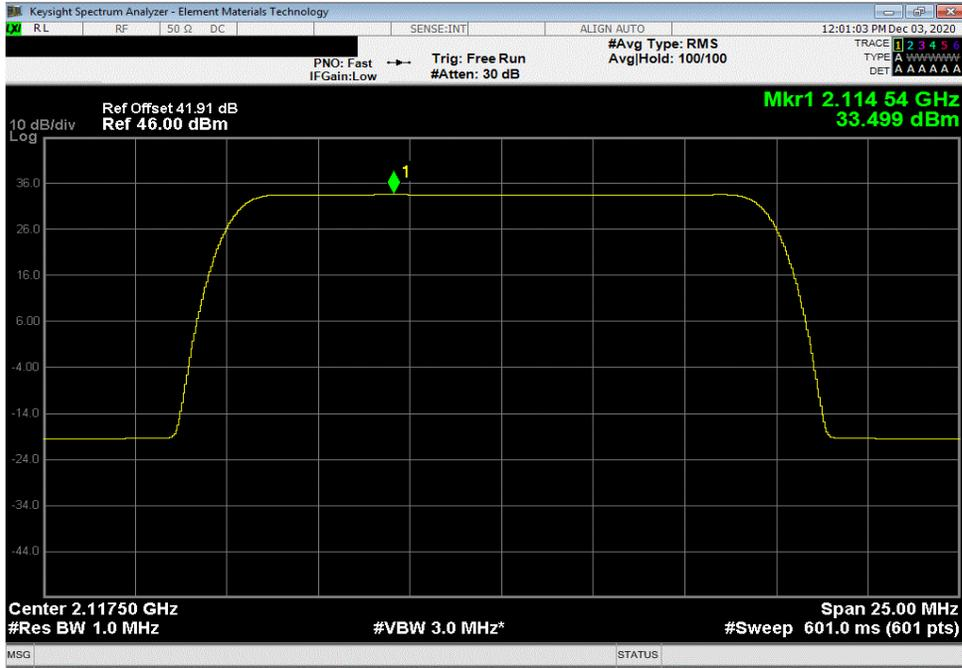
30 Watt Port 1, Band 1, 2110 MHz - 2155 MHz, 15 MHz Bandwidth, QPSK Modulation, Mid Channel 2132.5 MHz
