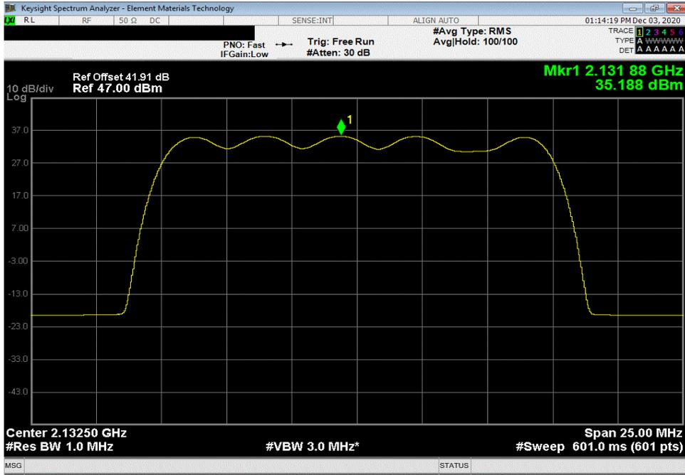
30 Watt Port 1, Band 1, 2110 MHz - 2155 MHz, 15 MHz Bandwidth, 16-QAM Modulation, High Channel 2147.5 MHz
