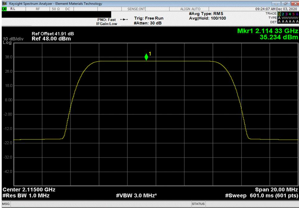
30 Watt Port 1, Band 1, 2110 MHz - 2155 MHz, 10 MHz Bandwidth, QPSK Modulation, Mid Channel 2132.5 MHz
