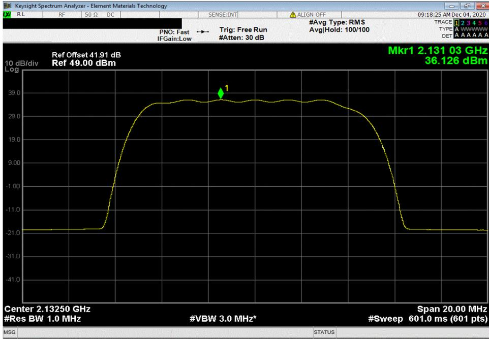
30 Watt Port 1, Band 1, 2110 MHz - 2155 MHz, 10 MHz Bandwidth, 16-QAM Modulation, High Channel 2150 MHz
