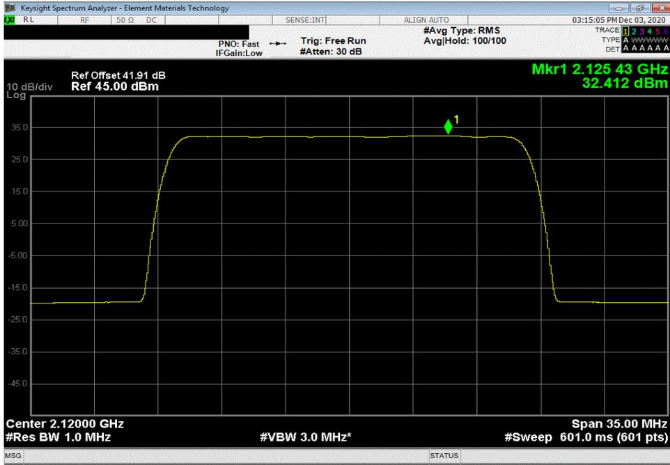
30 Watt Port 1, Band 1, 2110 MHz - 2155 MHz, 20 MHz Bandwidth, 64-QAM Modulation, Mid Channel 2132.5 MHz
