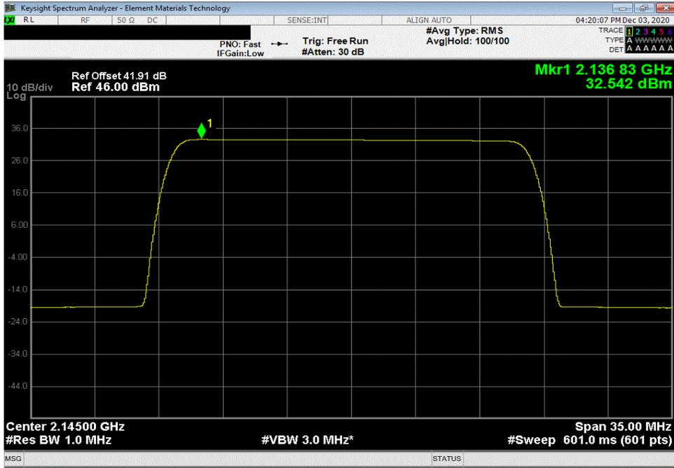
30 Watt Port 1, Band 1, 2110 MHz - 2155 MHz, 20 MHz Bandwidth, 16-QAM Modulation, Low Channel 2120 MHz
