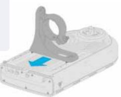
**3.7** Open the clamp with the swivel locking nut up out of the way. If your pole arm is smaller than 2.3/8" (60.3 mm), you will install a clamp insert set into the clamp. Clamp inserts are available in 1.25" sizes, and come as a set of two.
