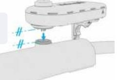
**6.4** Once plugged, rotate the UbiHub towards the pole to lock the NEMA connecter in place. Stop once the clamp is aligned with the pole.
