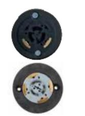
**6.3** Line up the NEMA plug on the UbiHub with the NEMA socket on the luminaire. The UbiHub should be slightly off-angle of the luminaire by 15 degrees once inserted.
