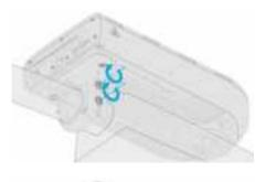
**B.** Then tighten the horizontal adjustment screws to 40 in-lbs torque using the 3/16" Hex bit driver.
