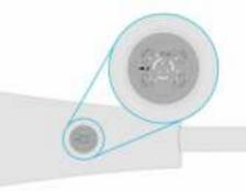
**A.** Use a screwdriver to remove the two screws. Unscrew the NEMA connector and lift then turn the NEMA connector until the N > is facing in the correct direction (away from the luminaire pole).
