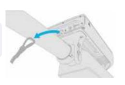
**6.9** Place the UbiHub APAI camera over the vertical adjustment bolts on the mounting clamp by toeing in the bottom and rotating upward into place. Ensure the camera cable is not crimped or pinched while installing onto the clamp.
