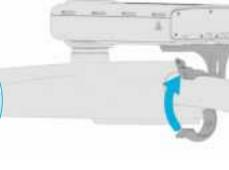
**6.6** Adjust the clamp vertically as necessary to ensure the device is parallel with the bottom of the luminaire to ensure there is no undue stress or strain on the NEMA socket.
