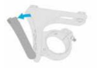
**3.5** Align the shuttles on the top of the clamp with the rail openings on the bottom of the UbiHub housing while still in the box. There is a single orientation for assembly.
