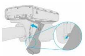
**6.10** Tighten the camera top screw to 15 in-lbs torque using the 3/16" Hex bit driver.
