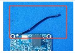
The antenna is internal antenna.
