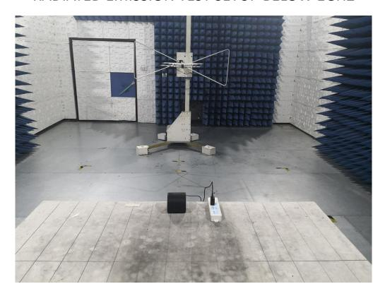
RADIATED EMISSION TEST SETUP ABOVE 1GHZ
