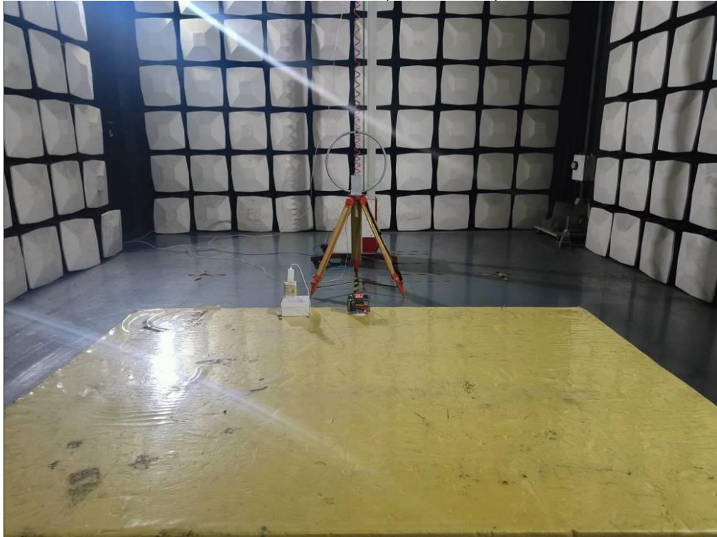
Test Photo Radiated emission (Below 30MHz)
