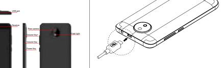
Batteries must be charged before they are first used. When charging, the charger should be close to the power socket and easy to unplug.
