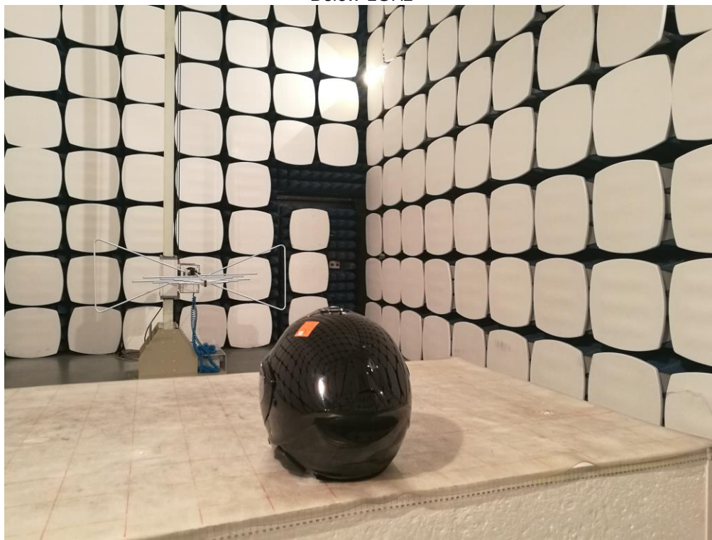
Radiated Emission Below 1GHz
