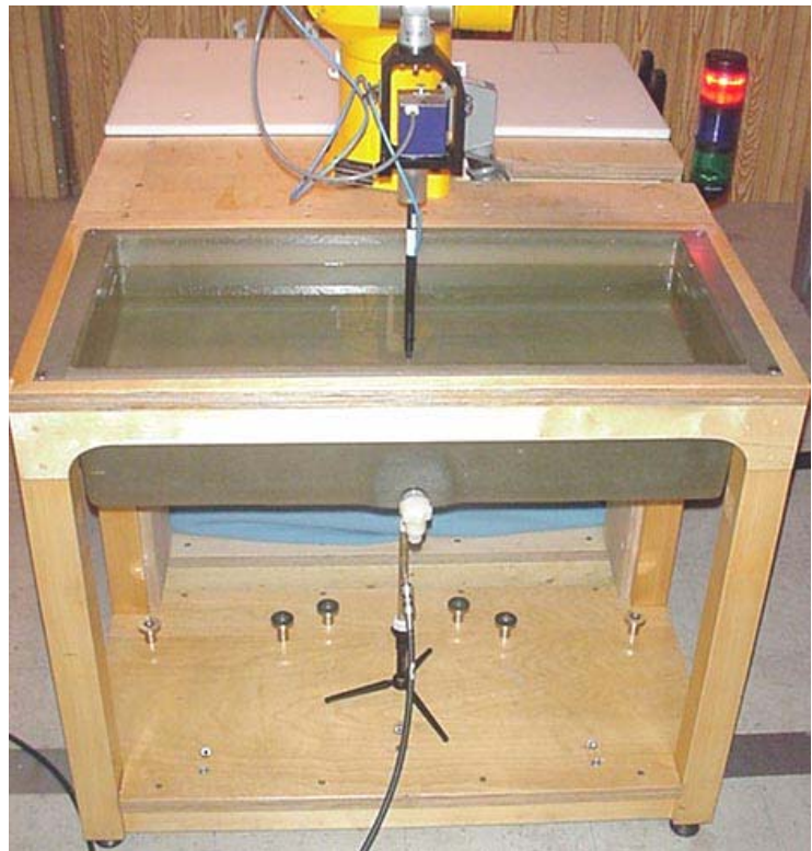
DASY4 SAR Measurement System with planar phantom & validation dipole
